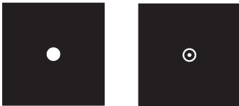
Figure 9-15 Comparison of Antialiased Points and Textured Point Sprites
