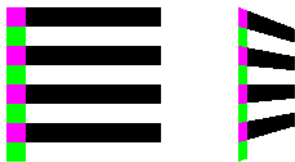
Figure 9-13 Repeating and Clamping a Texture
