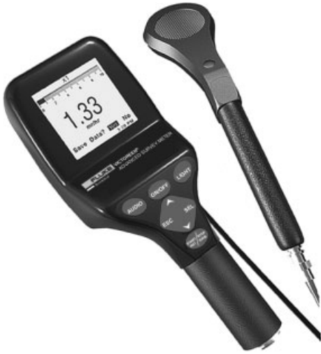
Fig. 10.11 Portable survey and count-rate meter with optional GM pancake probe. See text. (Courtesy Fluke Biomedical.)
