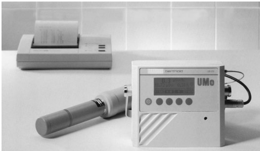
Fig. 10.7 Proportional-counter monitor for measuring dose and dose rate. See text. (Courtesy Berthold Technologies USA, LLC.)
