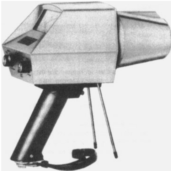
Fig. 10.5 Portable ionization-chamber survey meter (cutie pie). (Courtesy Victoreen, Inc.)
