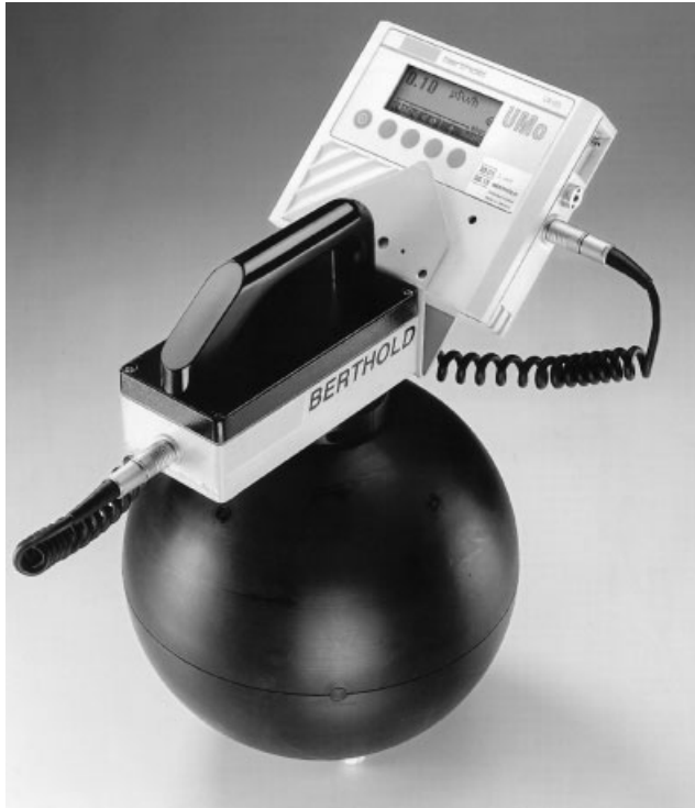
Fig. 10.44 Instrument for measuring neutron dose-equivalent rate. A ^3\text{He} proportional counter tube is located at the center of a polyethylene moderator sphere. The cylindrical tube has approximately equal height and diameter to minimize directional dependence
