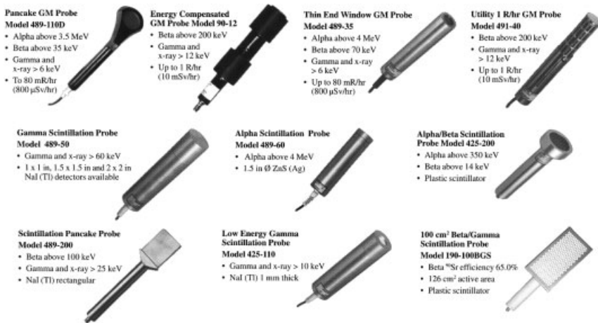
Fig. 10.12 Examples of Geiger–Mueller and scintillation probes with specifications. (Courtesy Fluke Biomedical.)
