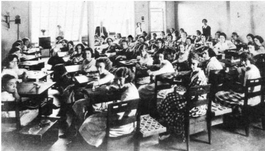
Fig. 13.6 A studio with radium dial painters, cir. 1920s. The proximity of the painted dials at the workers' sides and the supply of radium paint on their desks added an external gamma dose to the internal dose from the ingested radium. [From R. E. Rowland, Radium in Humans, a Review of U.S. Studies , Report ANL/ER-3, Argonne National Laboratory, Argonne, IL (1994).]
