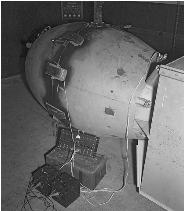
Fig. 4.3 The Nagasaki Fat Man plutonium implosion weapon shortly before its mission. Fat Man was 12 feet long, 5 feet in maximum diameter, and weighed 10,300 pounds when fully assembled (Sublette 2007). Photo courtesy Alan Carr, Los Alamos National Laboratory
