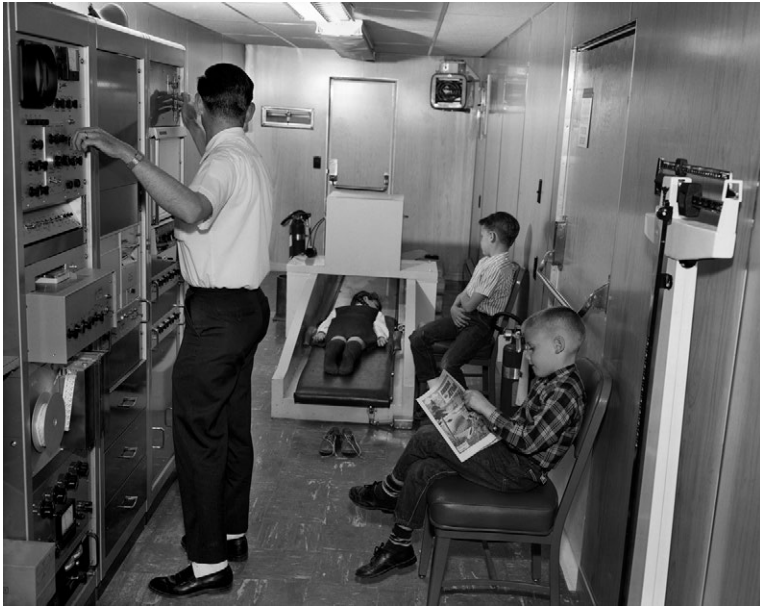
Figure 5.2 Interior of a truck-mounted radiation counter taken to schools to monitor radiation levels in children who lived near Hanford. This was a common practice in the mid 1960s.
