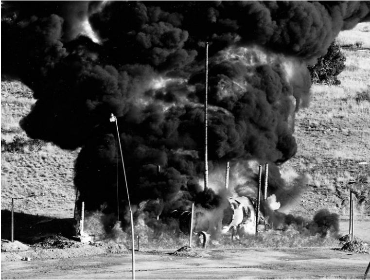
Figure 15.3 Burn test of transportation container at approximately 2000 °F (1100 °C) for thirty minutes. Source: US Department of Energy.
