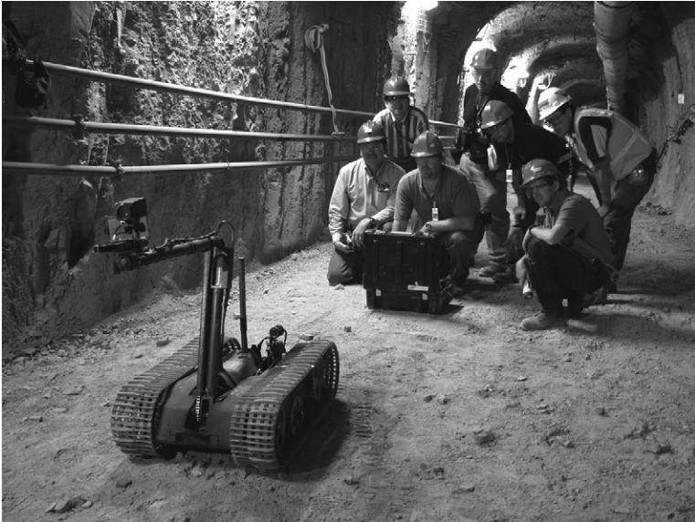
Figure 18.1 Robot equipped with video cameras in Exploratory Study Facility.
