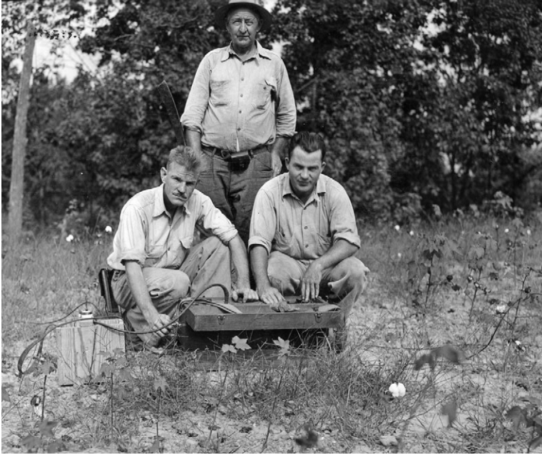
Figure 1.2 M. King Hubbert (on the left) setting up a resistivity instrument for a geophysical survey in Franklin Co., Alabama, September 22, 1934. Photograph by E.F. Burchard; courtesy US Geological Survey.
