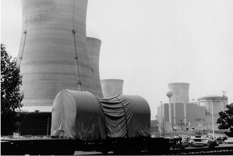
Figure 5.5 Damaged reactor core materials being shipped from Three Mile Island to Idaho National Laboratory.
