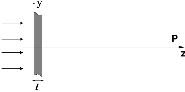
Figure 2.3. Light passes through a plane-parallel slab of thickness l with one face lying in the (x, y) -plane. The slab is uniformly filled with identically scattering particles. We determine the field at point P with coordinates (0, 0, z) .
