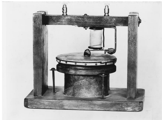
FIG. 1. Alexander Graham Bell's first telephone. Voice sounds were transmitted for the first time on June 3, 1875, over this gallows-shaped instrument. From Fagen, 1975.
