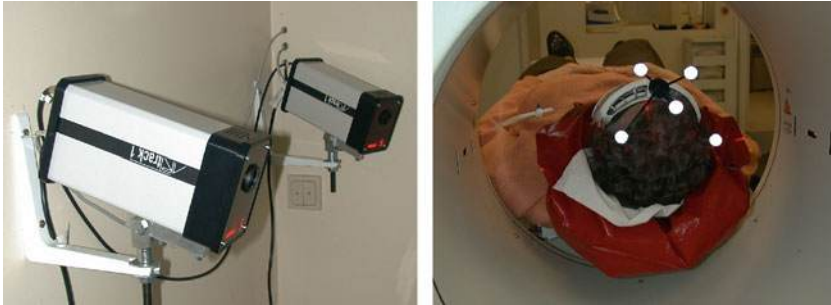
■ Fig. 8 Passive infrared motion tracking system monitoring the head motion of a patient while undergoing a PET examination. The system monitors the position of several spherical markers attached to a pair of goggles and delivers the positional information (specified by the six degrees of freedom of a rigid transformation relative to the reference position)
