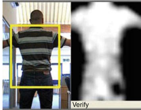
■ Fig. 2 CCTV and enhanced images of a passenger with a wallet in his hip pocket
