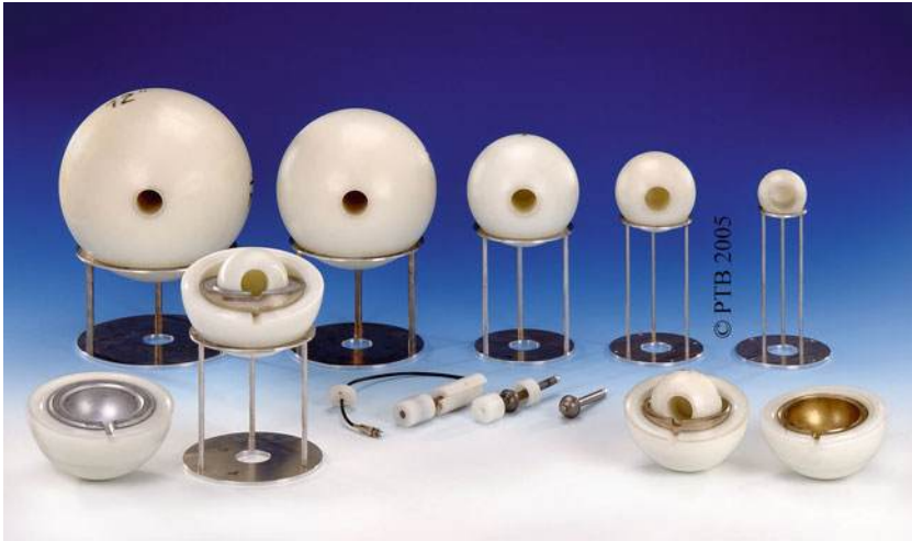
■ Fig. 5 Bonner sphere spectrometer NEMUS of the PTB with five of the ten polyethylene spheres in the back, a spherical 3 He proportional counter in the center, and parts of the modified spheres in the foreground left and right
