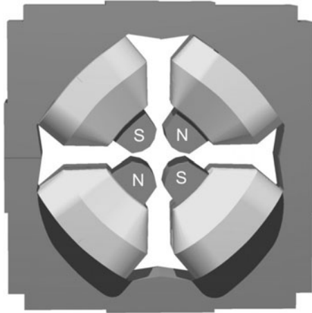
■ Fig. 9 Quadrupole magnet with four coils on an iron yoke with hyperbolic pole faces. In this example, an electron beam pointing into the image plane is focused vertically and defocused horizontally
