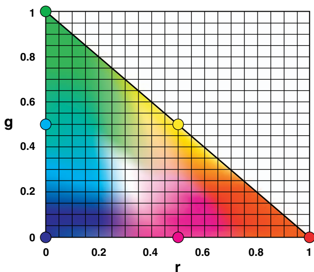
FIGURE 7.4 ► The color triangle here is filled with all the colors that can be obtained by mixing R, G, and B.
