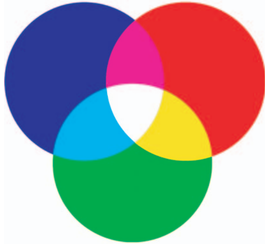
FIGURE 7.1 ► The most frequently adopted additive primary colors are R, G, and B.
