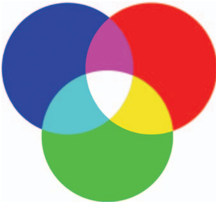
FIGURE 6.14 ► Three colored light beams, red, green and blue, overlap two at a time to form cyan, magenta and yellow. Colors at opposite ends of this diagram are complementary colors: red and cyan, green and magenta, blue and yellow. Where all three colors overlap the resulting color is white.
