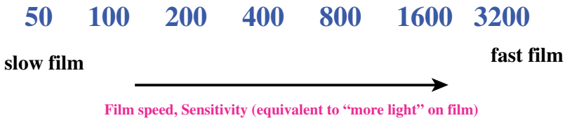
FIGURE 5.8 ► The film speed varies by factors of 2. A fast film has a large ISO number and needs less light, but has larger grain.
