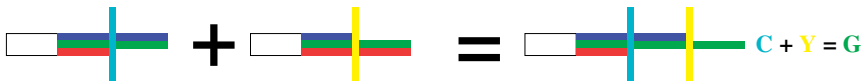
FIGURE 8.8 ▶ White light, coming from the left, can be for simplicity’s sake considered to have only RGB components. Each filter subtracts its complementary color. The cyan filter absorbs R (its complementary color) while transmitting B and G. Remember that additively B + G = C . Therefore, the B and G lights transmitted by the filter form C. The yellow filter absorbs B and transmits G and R. Again, additively G + R = Y , so a C filter transmits C light, a Y filter Y light. However, the combination of the two filters will only transmit G light. If we start from white light, we have R, G, and B. The cyan filter subtracts R and the yellow filter subtracts B, leaving only G to be transmitted. (R + G + B) - R - B = G .
