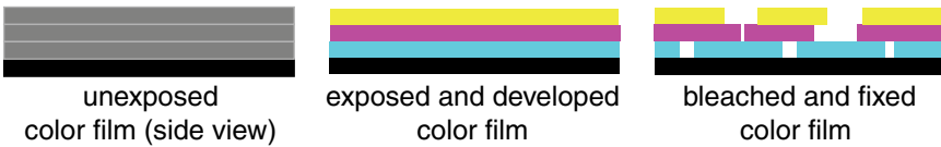
FIGURE 8.11 ► The unexposed film (left) appears gray. Once it has been exposed and developed the B, G, and R absorbing layers are colored. After bleaching and fixing, the silver halide crystals are removed, and only the color layers remain but only in the appropriate places to produce a negative of the image. Where only the cyan layer is present, the image will be printed red, and so on.
