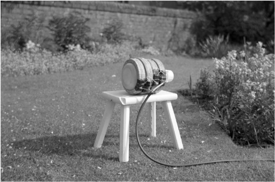
Experimental set-up of an early high precision search for an anisotropy of inertia.
