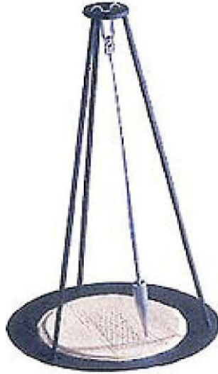
FIGURE 2. The Galileo/Huygens pendulum. The small oscillations are remarkably regular and periodic. When counting the number of oscillations of the pendulum, we measure a time interval, thus realizing a clock. The shorter the pendulum period, the greater number of oscillations in a time interval and the more precise will be the determination of this time interval. Modern clocks use electromagnetic signals where the period is 10^{10} to 10^{15} times shorter than the typical 1 second period of a pendulum.
