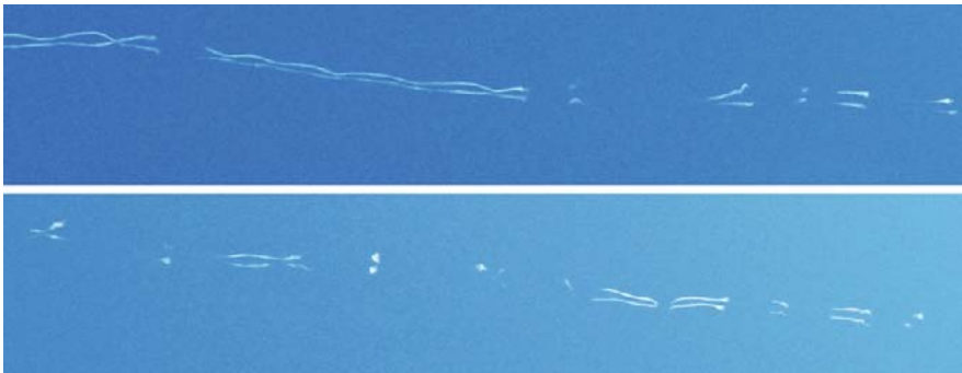
Fig. 5. Breakdown via the so-called Crow instability of a pair of vortex tubes trailing an aircraft. What is seen is the interaction of the vortices with the condensation trail from the jet engines; the lower half of the picture continues the upper half on the right. From http://commons.wikimedia.org/wiki/File:The_Crow_Instability.jpg .
