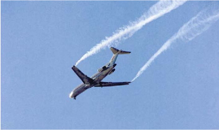
Fig. 4. This picture shows the wing-tip vortices which are associated with the circulation generating lift coming off the wings of a Boeing 727 aircraft. They were made visible by smoke generators installed on the tips of the aircraft wings. (NASA photograph number ECN-3831.)
