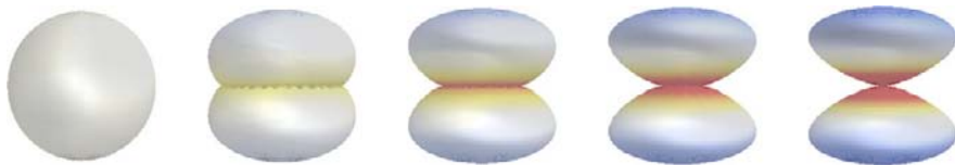
Fig. 2. Illustration of the rotating balloon thought experiment. As the lasso contracts, conservation of circulation implies that the velocity along the waist increases (indicated by red colors) while the velocity on the outer lobes decreases (indicated by blue colors).
