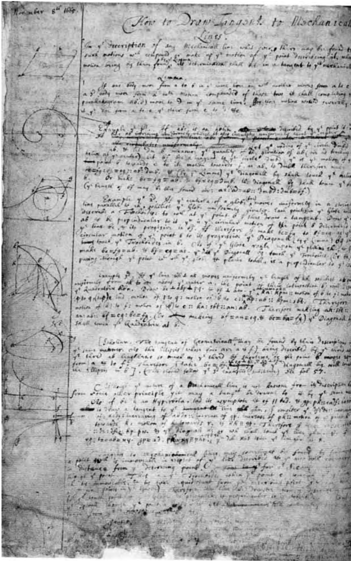
Figure 6. Newton’s early work (November 1666) on tangents to ‘mechanical lines’ (i.e. transcendental plane curves). His technique consisted in conceiving curves as generated by motion and resolving motion into components. Source: [9], vol. 1, 378.
