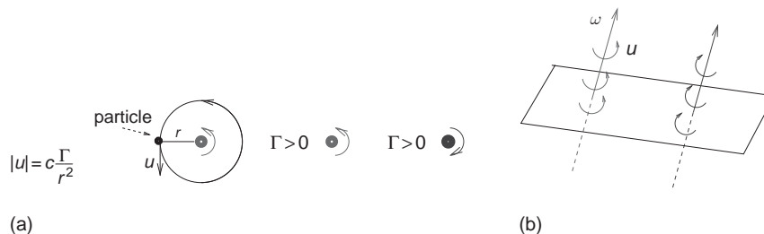
Figure 4 (a) Advected by the velocity field of one point vortex, a test particle follows a circular orbit, with a speed proportional to the absolute value of the vortex circulation and inversely proportional to the square of its distance from the vortex. (b) Straight vortex lines.
