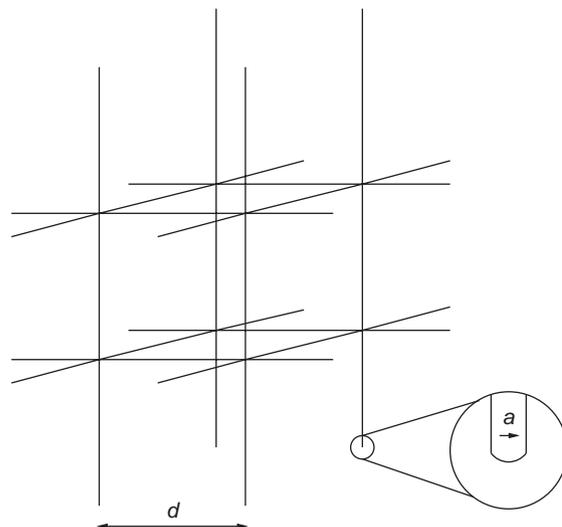
**Figure 1** A periodic structure composed of infinite conducting wires arranged in a simple cubic lattice. Provided the factor  $a/d$  is small enough, the structure responds to incident electromagnetic waves as a plasma of very heavy charged particles.
