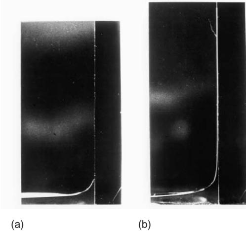
**Figure 16** Distilled water in wedges formed by acrylic plastic plates;  $g > 0$ . (a)  $\alpha + \gamma > \pi/2$ ; (b)  $\alpha + \gamma < \pi/2$ . Reproduced from P Concus and R Finn, “On Capillary Free Surfaces in a Gravitational Field” in *Acta Math* 132 (1974) 207–223 with permission of Institut Mittag-Leoffler.
