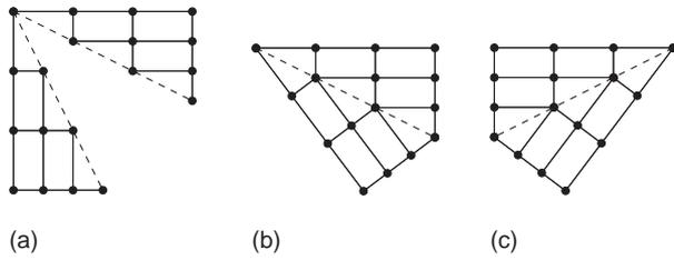
**Figure 2** Formation of phase boundaries in a single crystal. (a) The upper right half of the lattice deforms into phase I with the constant deformation gradient  $U_1$ , the lower left half of the lattice deforms into phase II with constant deformation gradient  $U_2$ . (b) An additional rotation is needed to accomplish a continuous deformation, see formula [3]. (c) A different configuration with a different orientation of the interface. (Sketch not to scale.)
