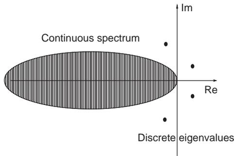
Figure 11 Spectrum for the flow around an obstacle.
