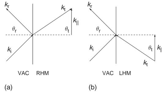
**Figure 4** Illustration of Snell's law at an interface between two media with (a) positive refractive index (VAC/RHM) and (b) negative refractive index (VAC/LHM). The arrows indicate the wave vectors and the energy flow is opposite to the wave vector in the negative index medium.
