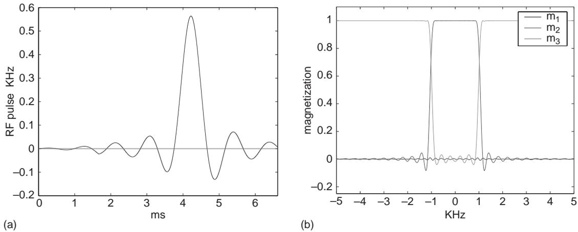
**Figure 2** A selective  $90^\circ$  pulse and profile designed using the inverse scattering approach. (a) Profile of a  $90^\circ$  inverse-scattering pulse. (b) The magnetization profile produced by the pulse in (a).
