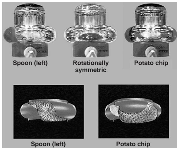
**Figure 10** Symmetry breaking in exotic container,  $g = 0$ . Below: calculated presumed global minimizer (spoon) and local minimizer (potato chip). Above: experiment on Mir: symmetric insertion of fluid (center); spoon (left); potato chip (right). This is a grayscale version of a color figure reproduced from *Journal of Fluid Mechanics*, 224: 383–94, (1991) with permission of Cambridge University Press.
