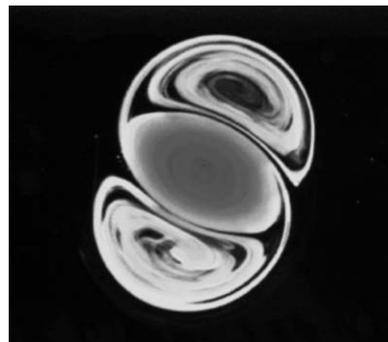
**Figure 13** A tripolar vortex structure as observed in a rotating stratified fluid. Reproduced from van Heijst GJF, Kloosterziel RC, and Williams CWM (1991) Laboratory experiments on the tripolar vortex in a rotating fluid. *Journal of Fluid Mechanics* 225: 301–331, with permission from Cambridge University Press.
