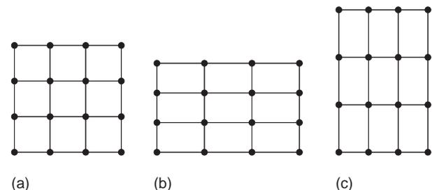
**Figure 1** Two-dimensional cartoon of a cubic to tetragonal phase transformation in a single crystal: (a) a cubic lattice, (b) and (c) tetragonal variants which are stretched in directions  $e_1$  and  $e_2$ , respectively. (Sketch not to scale.)
