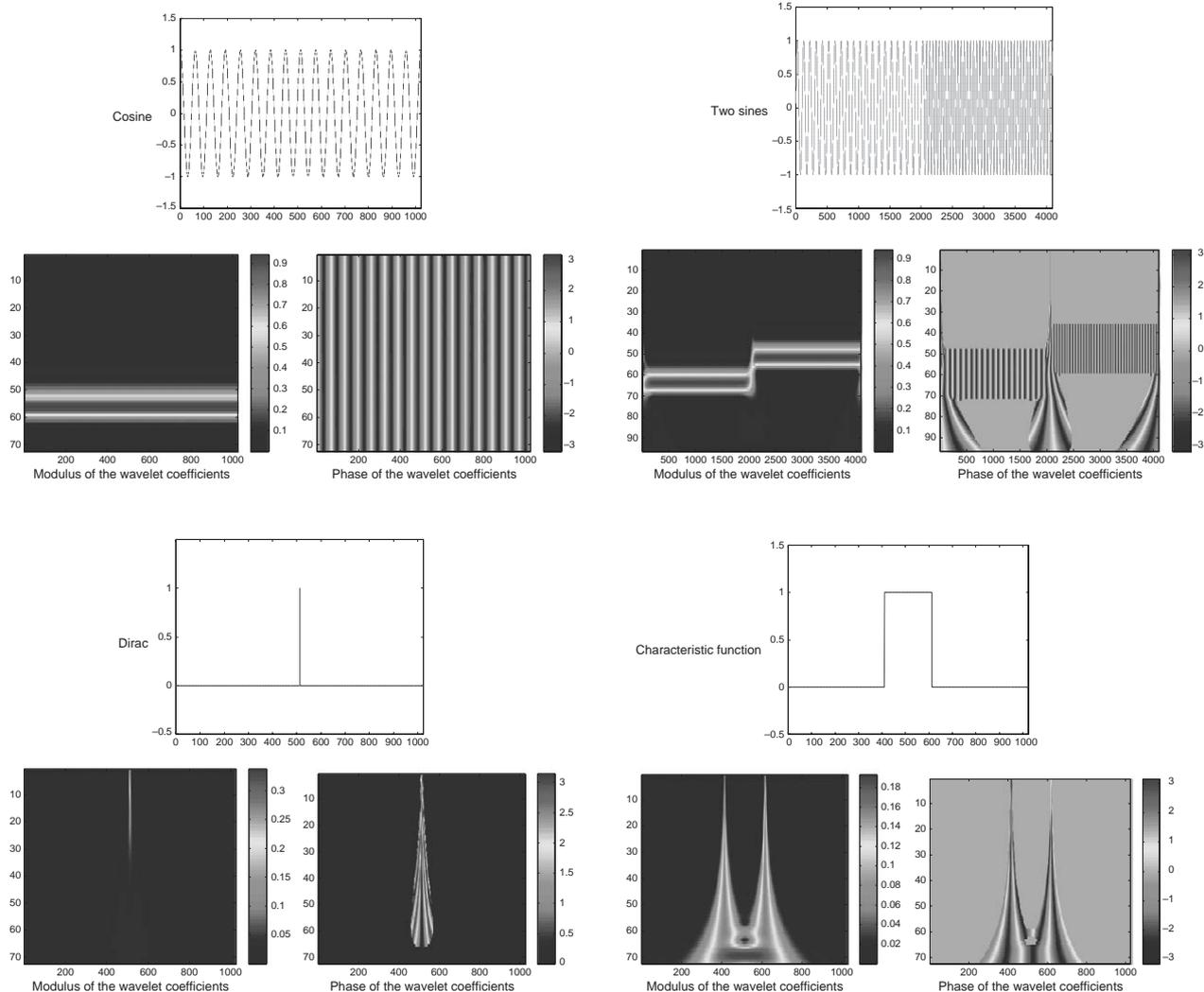
**Figure 1** Examples of a one-dimensional continuous wavelet analysis using the complex-valued Morlet wavelet. Each subfigure shows on the top the function to be analyzed and below (left) the modulus of its wavelet coefficients and below (right) the phase of its wavelet coefficients.
