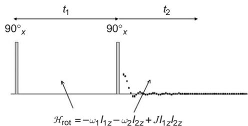
**Figure 4** RF pulse scheme used for COSY experiment.
