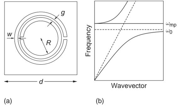
**Figure 2** (a) The split-ring resonator structure. The structure is planar with an internal radius  $R$ . The metal rings are of width  $w$  and are separated by a spacing  $g$ . (b) Generic dispersion relationship,  $\omega$  vs.  $k$ , for a resonant structure with an isotropic effective permeability as in eqn [15].
