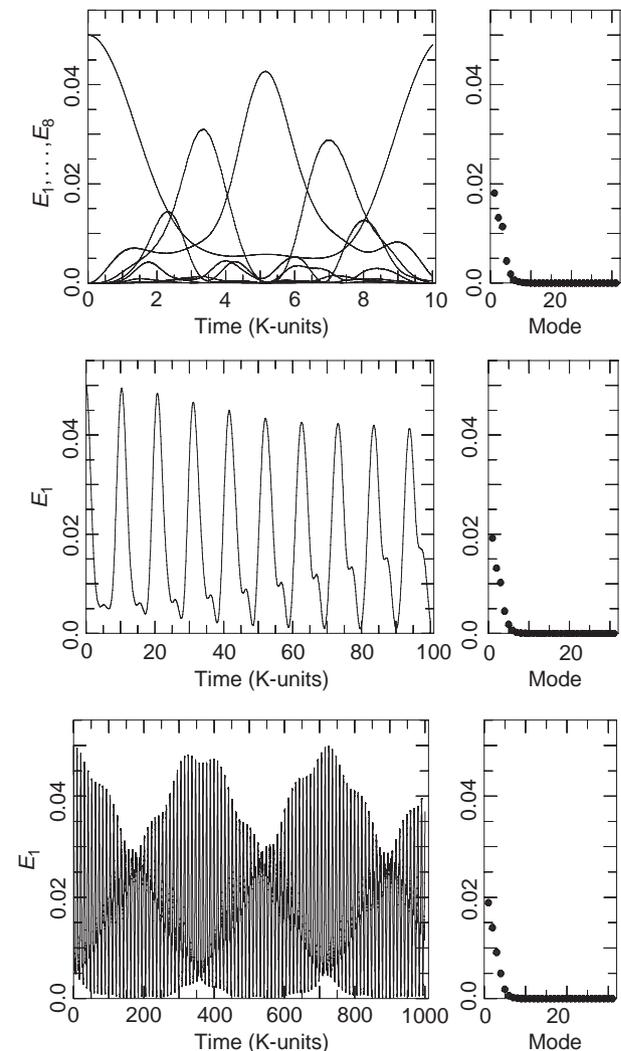
**Figure 1** The FPU paradox: normal-mode energies  $E_j$  versus time (left) and energy spectrum, namely time average of  $E_j$  versus  $j$  (right) for three different timescales. The energy, initially given to the lowest-frequency mode, does not flow to the high-frequency modes within the accessible observation time. Here,  $N = 32$  and  $E = 0.05$ .
