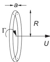
**Figure 11** Self-induced motion of a vortex ring.
