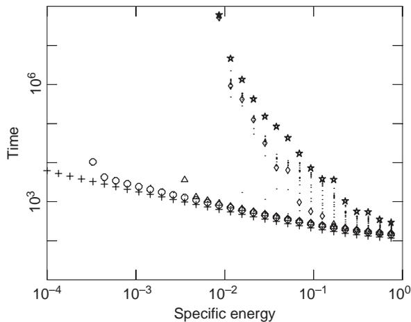
**Figure 6** Time needed to form a packet versus specific energy for the FPU model (bottom) and the corresponding Toda model (top). Different symbols refer to packets of different width. The existence of two timescales below a critical specific energy in the FPU model is exhibited.
