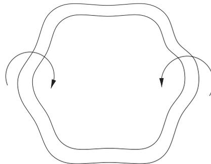
**Figure 12** Sketch. Onset of azimuthal vortex ring instability.
