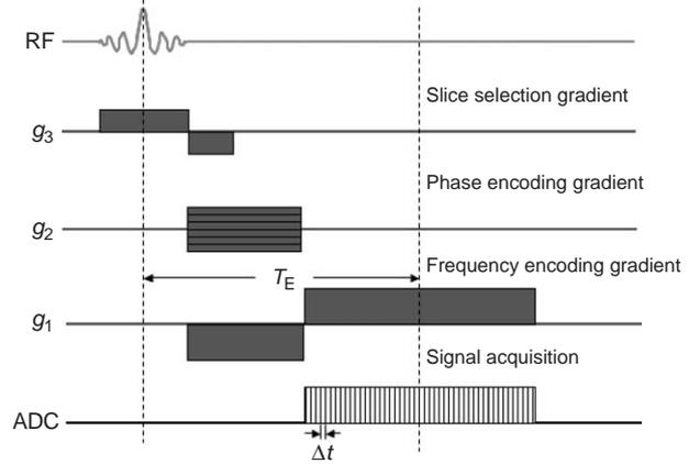
**Figure 3** Pulse timing diagram for spin-warp imaging. During the positive lobe of the frequency encoding gradient, the analog-to-digital converter (ADC) collects samples of the signal produced by the rotating transverse magnetization.
