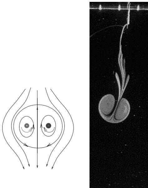
**Figure 11** Test-particle trajectories: on the left, theoretical trajectories, from the point-vortex model; on the right, a top view of a laboratory experiment in stratified flows. Reproduced from van Heijst GJF and Flor JB (1989) Dipole formation and collisions in a stratified fluid. *Nature* 340: 212–215, with permission from Nature Publishing Group.
