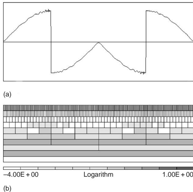
**Figure 8** (a) Nonlinear approximation  $f^N$  of the function  $f$  in Figure 5 reconstructed from the 64 largest wavelet coefficients using quintic splines wavelets, (b) retained wavelet coefficients  $\log_{10} |\tilde{f}_{j,i}|$  for  $i=0, \dots, 2^j - 1$  and  $j=0, \dots, J-1$ .
