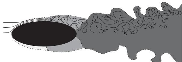
**Figure 2** Illustration of a flow past an object, with a laminar boundary layer (light gray), a turbulent boundary layer (medium gray), and a turbulent wake (dark gray).
