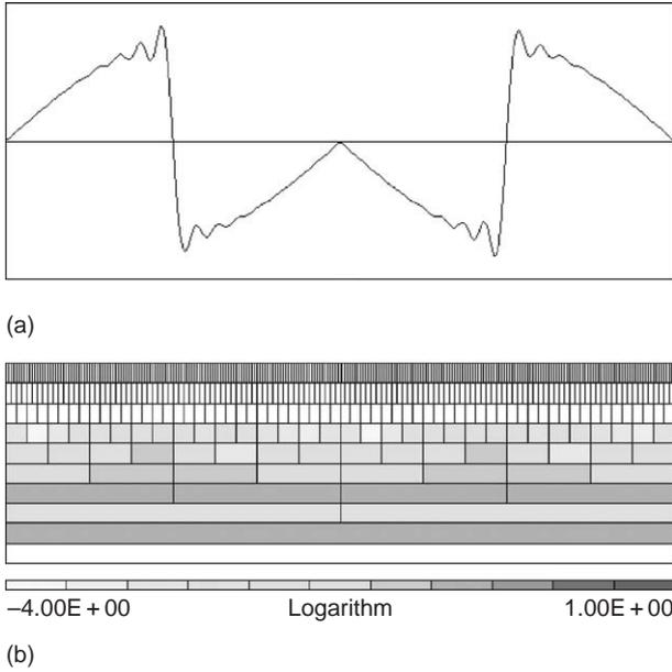
**Figure 6** (a) Linear approximation  $f_J$  of the function  $f$  in Figure 5 for  $J=6$ , reconstructed from 64 wavelet coefficients using quintic splines wavelets and (b) corresponding wavelet coefficients  $\log_{10} |\tilde{f}_{j,i}|$  for  $i=0, \dots, 2^j - 1$  and  $j=0, \dots, J-1$ . Note that the coefficients for  $J > 5$  have been set to zero.
