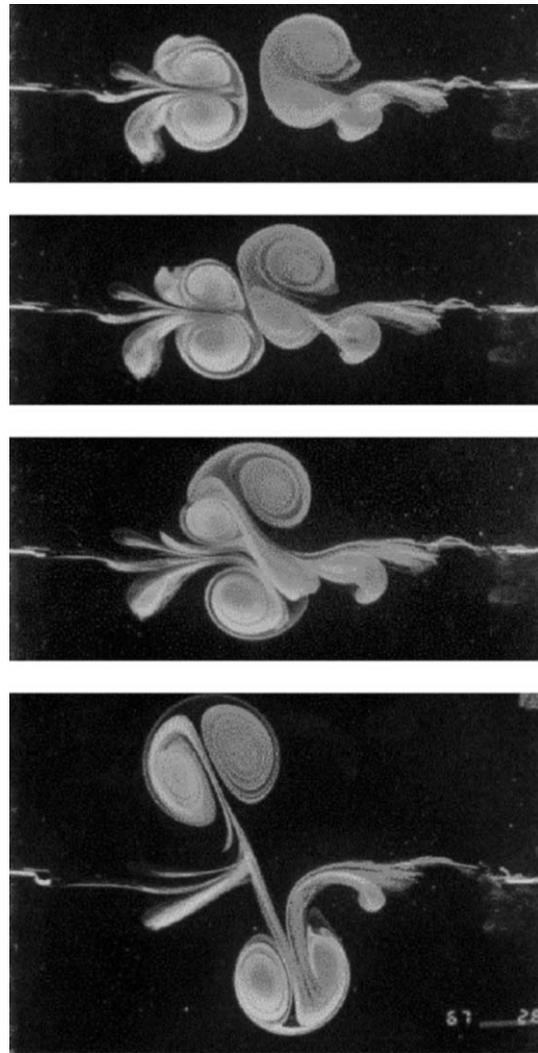
**Figure 12** A frontal collision of two dipoles as observed in a stratified fluid: after a so called “partner-exchange” two new dipoles are formed. Reproduced from van Heijst GJF and Flor JB (1989) Dipole formation and collisions in a stratified fluid. *Nature* 340: 212–215, with permission from Nature Publishing Group.
