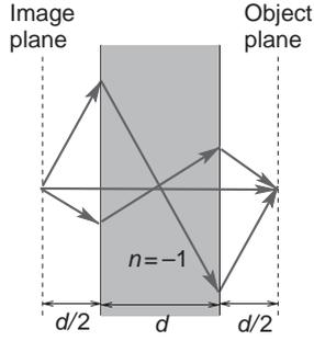
**Figure 5** Steady-state passage of rays (representing the energy flow) of light from vacuum through a slab made of a LHM with  $n = -1$ . The slab acts as a lens mapping a point on the image plane to a point on the object plane.
