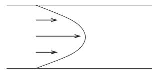
**Figure 3** Poiseuille flow with the trivial solution.
