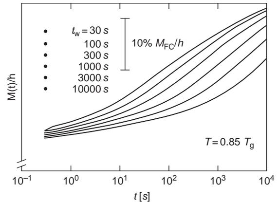
**Figure 2** ZFC magnetization in an aging experiment. The curves, from bottom to top, correspond to increasing waiting times. Reproduced from Norblad P and Svendlidh P (1997) Experiments in spin glasses. In: Young AP (ed.) *Spin Glasses and Random Fields*. Singapore: World Scientific, with permission from World Scientific Publishing Co. Pte Ltd.
