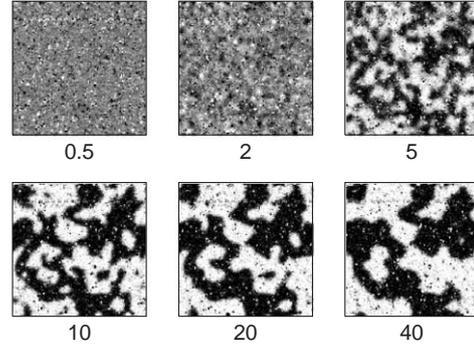
**Figure 1** Time evolution of  $\psi$  in model [1] in 2D with system length = 128. The numbers are the times after quenching. Noise is added, but is not essential for large patterns or in the late stage. Reproduced with permission from Onuki A (2002) *Phase Transition Dynamics*. Cambridge, UK: Cambridge University Press.
