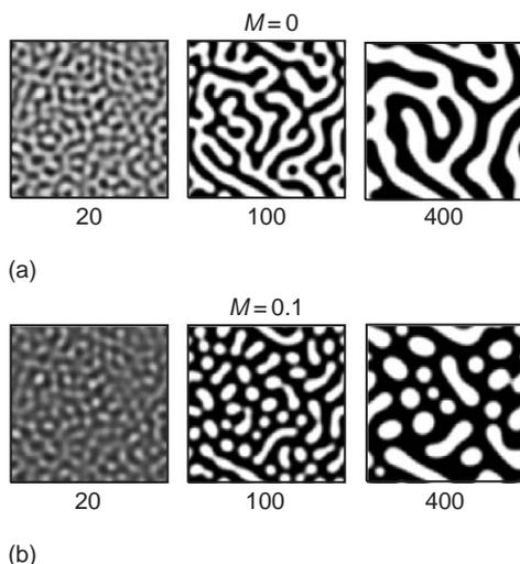
**Figure 2** Time evolution of  $\psi$  in model [23] in 2D with system length = 128 without thermal noise: (a)  $M=0$  and (b)  $M=0.1$ . The numbers are the times after quenching. Reproduced with permission from Onuki A (2002) *Phase Transition Dynamics*. Cambridge, UK: Cambridge University Press.
