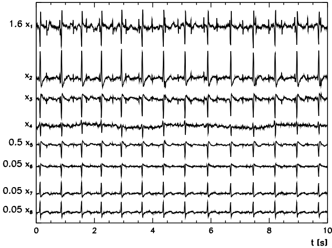
Fig. 6.16 Electro-cardiogram of a pregnant woman. The relatively weak and noisy signal of the child's heartbeat, visible in signals x_1 , x_2 , and x_3 , mixes with the signal of the mother's heartbeat (Example adapted from [56] based on data from [57])
