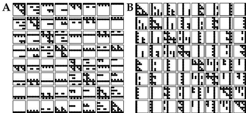
Fig. 3.1 Strassen's multiplication of 8 \times 8 matrices. The diagrams show the elements of A and B which are accessed in memory in order to form the elements of C . For example, to get the C_{18} element ( upper right corners ) we need A_{1k} ( 1 \leq k \leq 8 ) and B_{k8} ( 1 \leq k \leq 8 ) as in classical multiplication (3.1), but a different pattern for other elements
