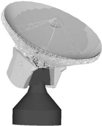
Fig. 2.27. Deformation of antenna structure
