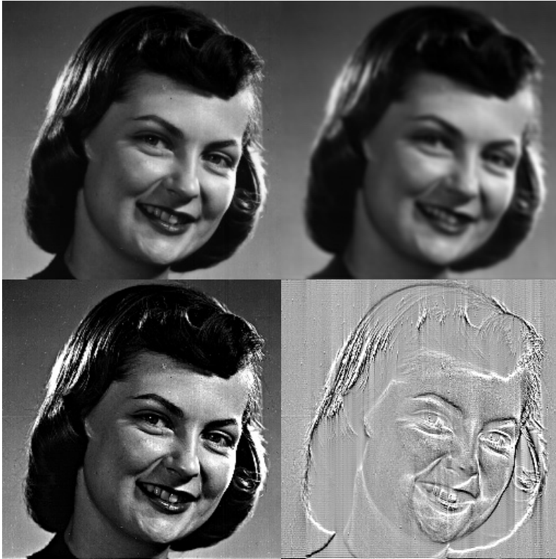
Figure 12.6.2. Fourier processing of an image. Upper left: Original image. Upper right: Blurred by low-pass filtering. Lower left: Sharpened by enhancing high frequency components. Lower right: Magnitude of the derivative operator as computed in Fourier space.
