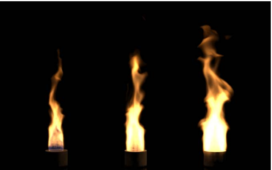
Figure 22.5. The density ratio of the unburnt to burnt gas is increased from left to right, illustrating the effect of increased expansion. (See also color figure, Plate 22.)
