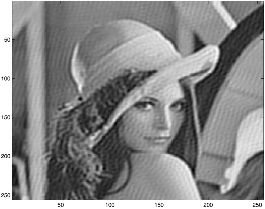
Figure 11.9. Linear deconvolution applied to Figure 11.8.
