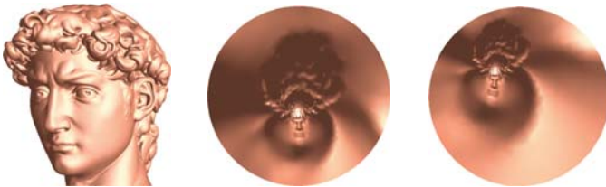
Fig. 1. According to Riemann Mapping theorem, a topological disk can be conformally mapped to the unit disk. Two such conformal maps differ by a Möbius transformation of the unit disk
