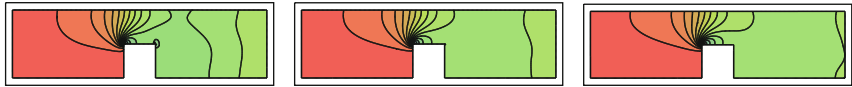
Fig. 7 Pressure contours for the flow in the channel with an obstruction for Reynolds numbers Re = 100, 200, 400 and L = 4
