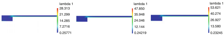
Fig. 5 First eigenvalue of the conformation tensor for We = 18, 30 and 33.5
