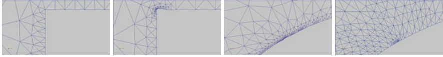
Fig. 4 Detection of genuine geometric singularities. Evolution of the initial upper-left corner of \Gamma_s (see top of Figs. 1 and 3): snapshots of iterations 0, 1, 160 and 190. The adaptive SQP method is able to sort out whether geometric singularities are genuine to the problem or just due to lack of numerical resolution and to coarsen overrefined regions of the computational grid
