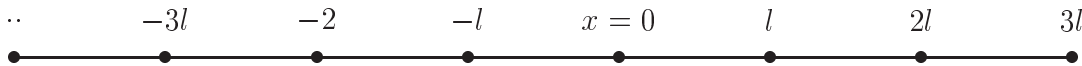
Figure 10.2: One-dimensional walker which can jump either to the left or to the right. Every step has length \Delta x = l .
