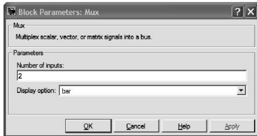
FIGURE 2.6 The parameter window for the Simulink block MUX.
