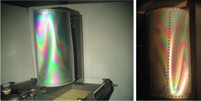
Fig. 23. Optical effect distributions: a model with 3 stringers (left), a model with 5 stringers (right)
