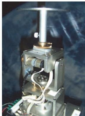
Fig. 2. Rotational motion simulator using z-y-z Euler angles.
