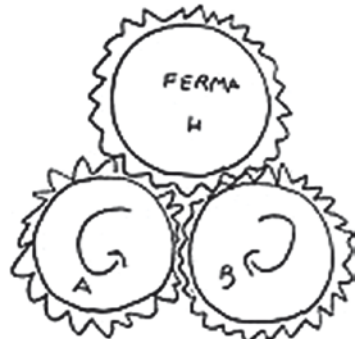
Fig. 11.11 If the A wheel turns left, the B wheel turns right. How can the other wheel turn? It cannot turn right because of the B wheel and it cannot turn left because of the A wheel. Hence they cannot turn
