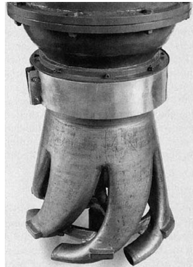
Prototype of a water turbine built according to EULER's proposals
