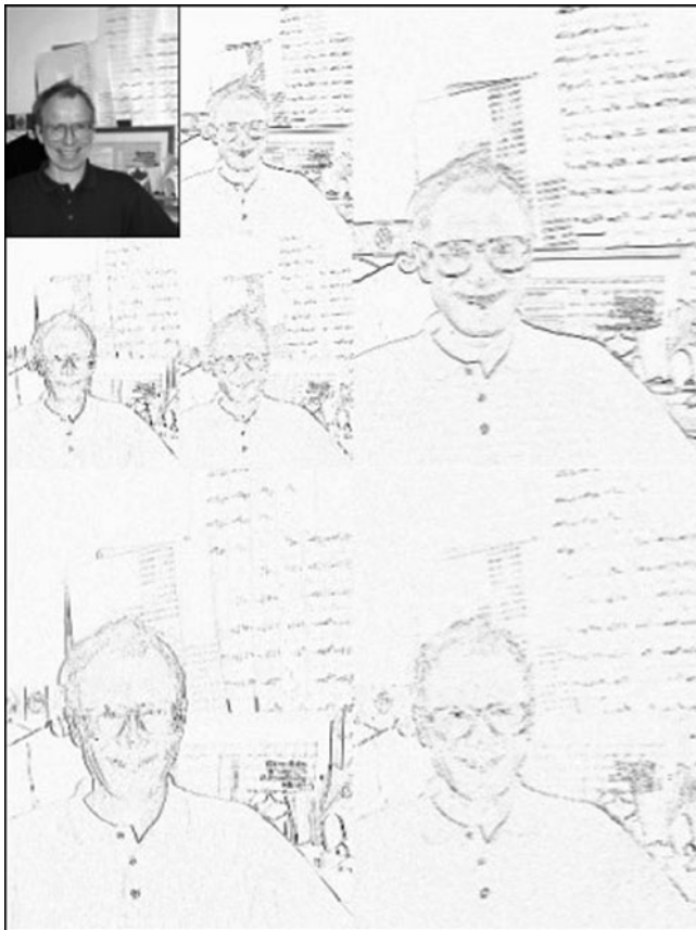
Fig. 8.5 An example of Fig. 8.4: n = 2 Jorgensen. Jorgensen’s picture after level 2 wavelet decomposition. Notice that The average, horizontal, diagonal and vertical details are captured clockwise. Also, the average detail is decomposed one more time since level 2 decomposition was done
