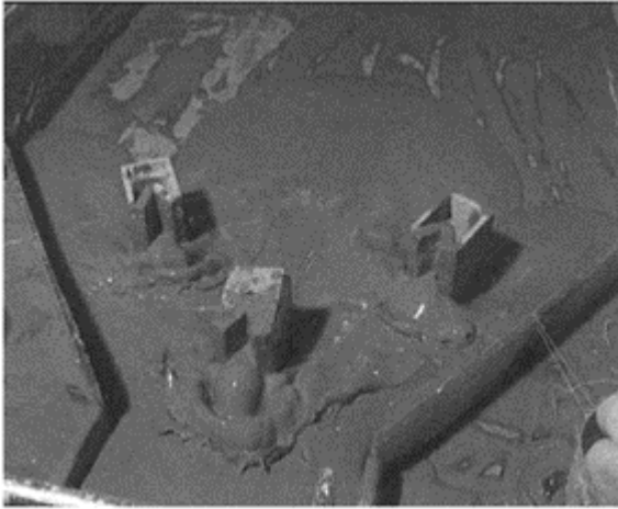
Figure 3. M-30-d1 type mudflow breakers.
