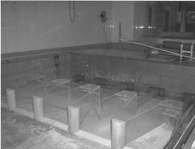
Figure 3. Photograph showing SWLCC model setup in the laboratory.
