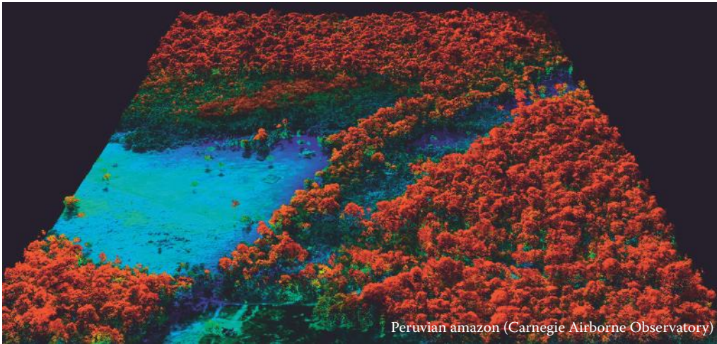
FIGURE 12.8 Example of airborne Lidar for mapping the three-dimensional properties of canopy surfaces (Adapted with permission from Macmillan Publishers Ltd., Tollefson, J., Nature 461:1048, copyright 2009.)
