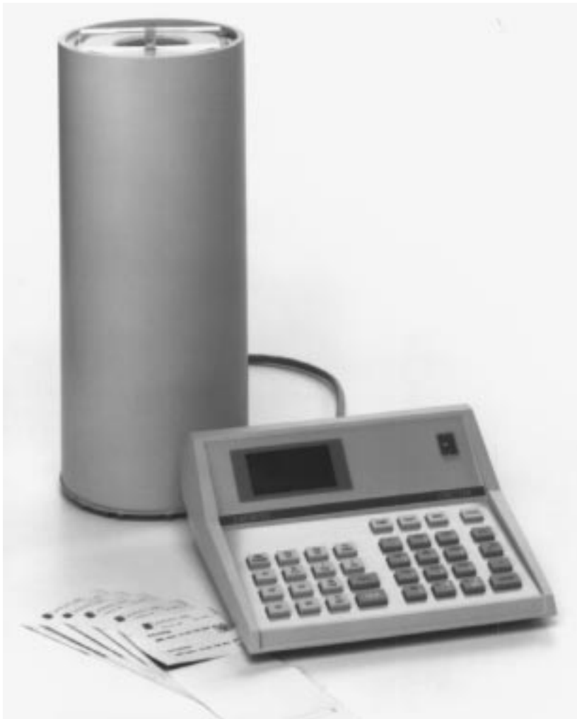
FIGURE 65.16 A well-type ionization chamber used for the assay of single radionuclides in nuclear medicine [26].
