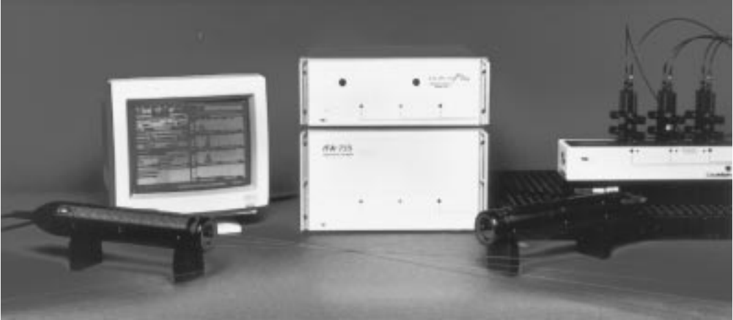
FIGURE 29.28 Three-component LDV system with fiber-optic probes.
