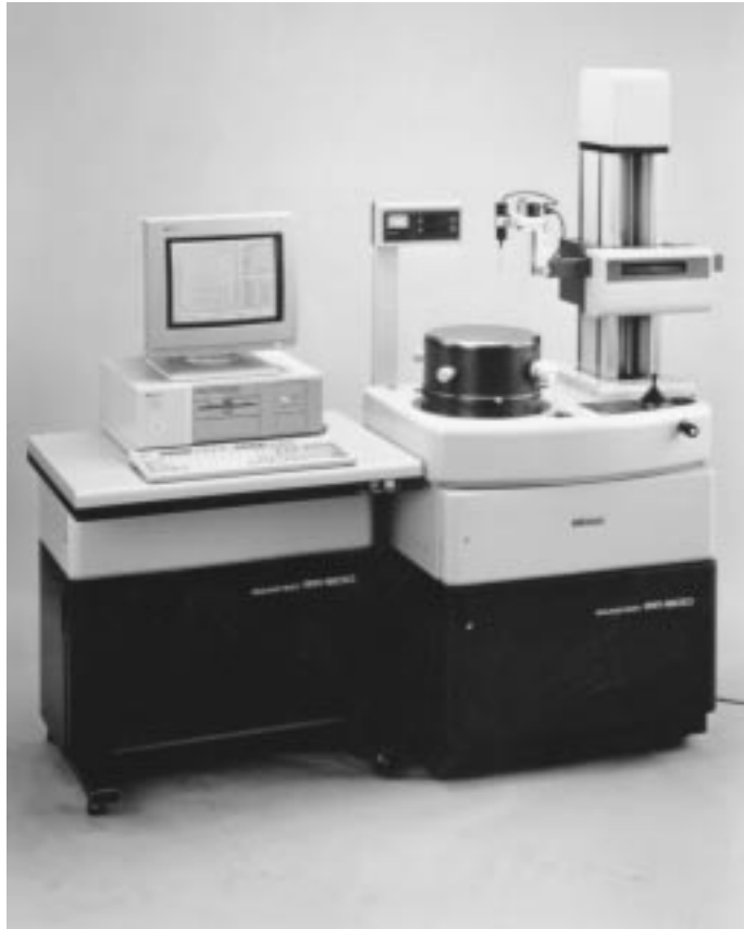
FIGURE 6.60 Fully automatic form measuring machine RA-600 (Courtesy of MITUTOYO/MTI Corporation).
