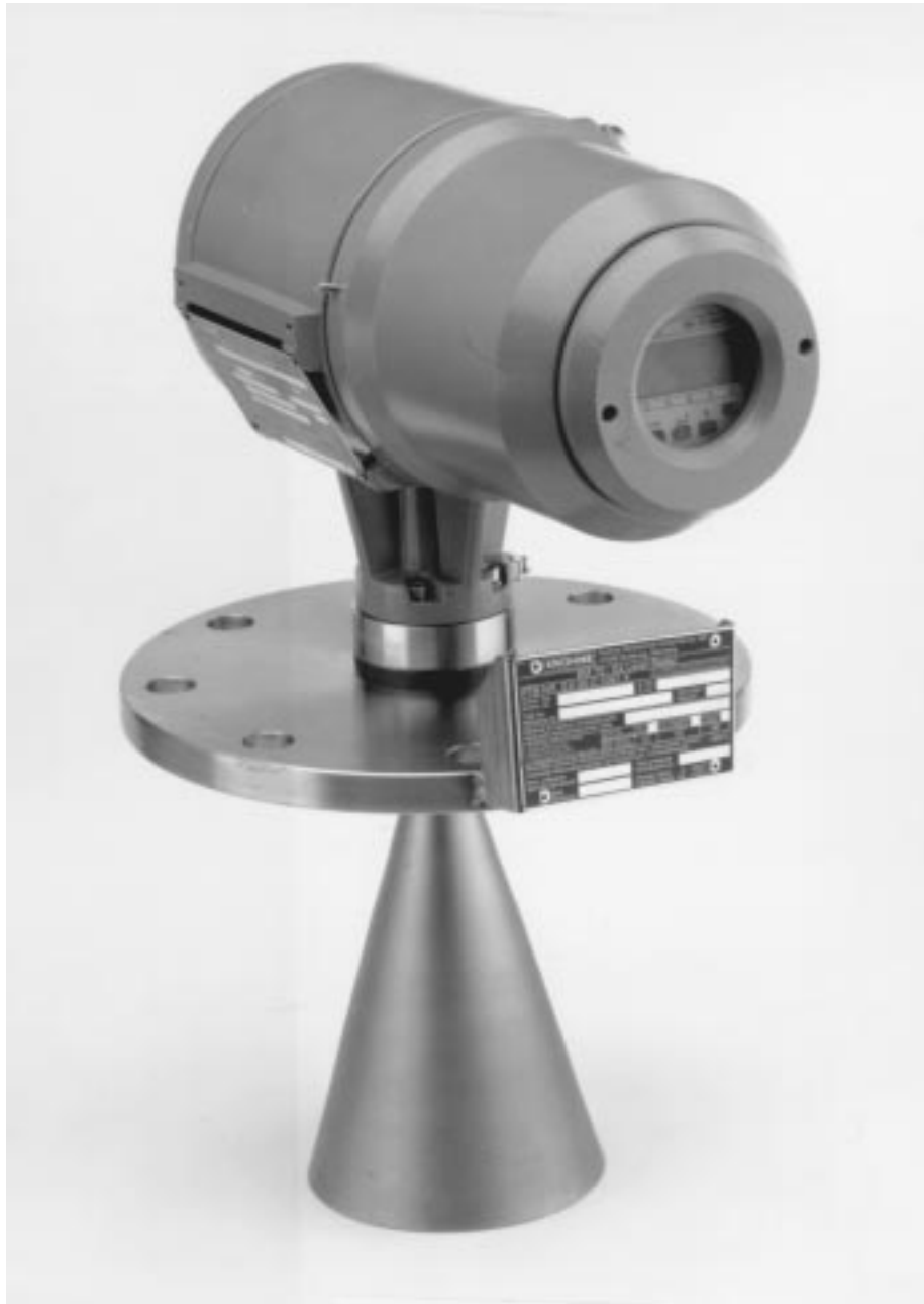
FIGURE 11.8 Design of a compact industrial level radar system. The converter above the flange includes the complete microwave circuitry, signal processing stages, microprocessor control, display, power supply, and output signal [6].
