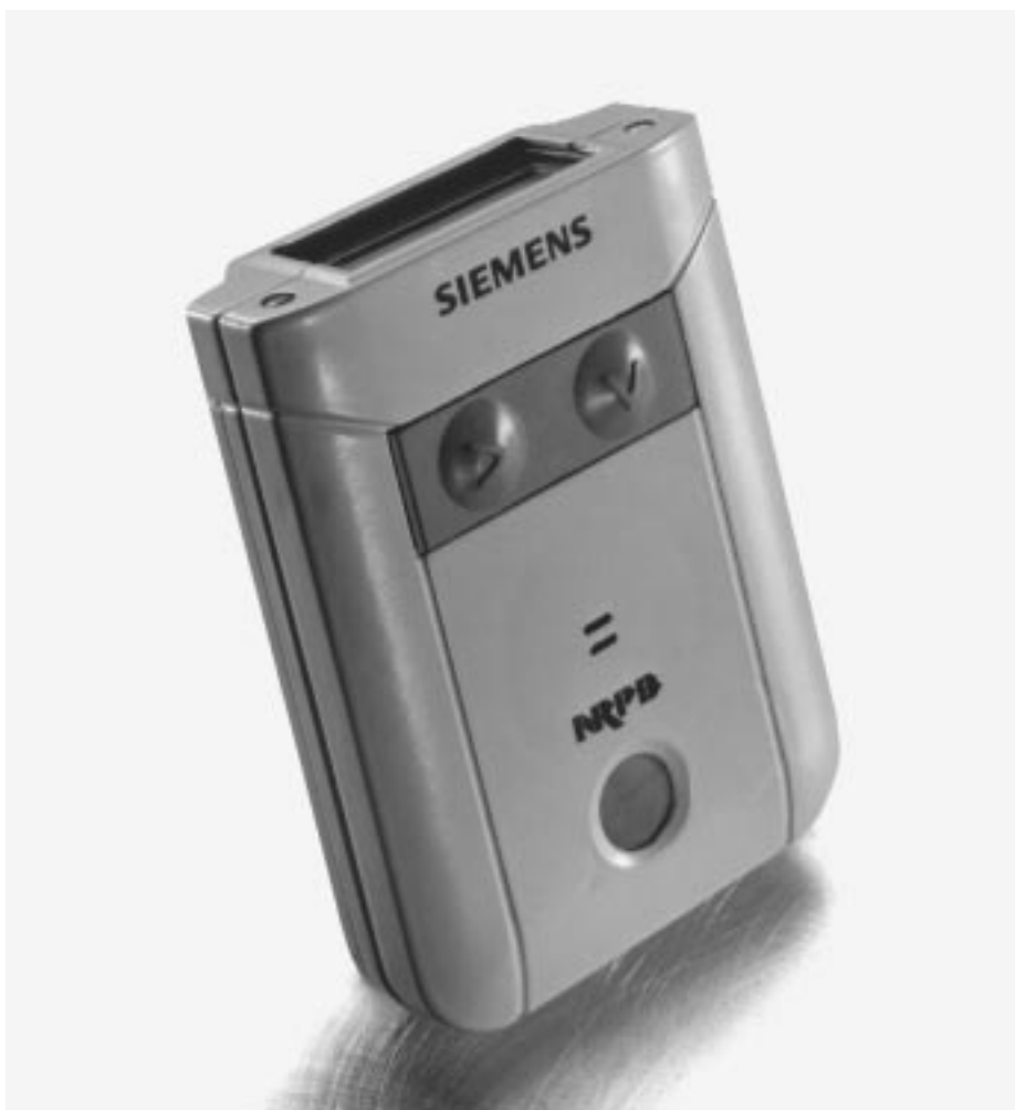
FIGURE 69.6 Electronic personal dosimeter. (Courtesy of Siemens Medical Systems, Inc.)
