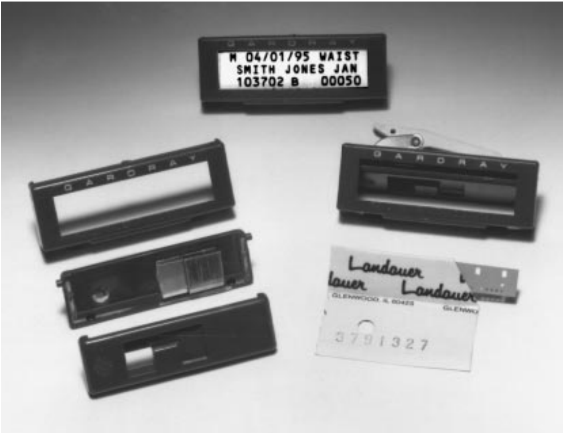
FIGURE 69.4 Film badge for personal dosimetry. (Courtesy of Landauer, Inc.)
