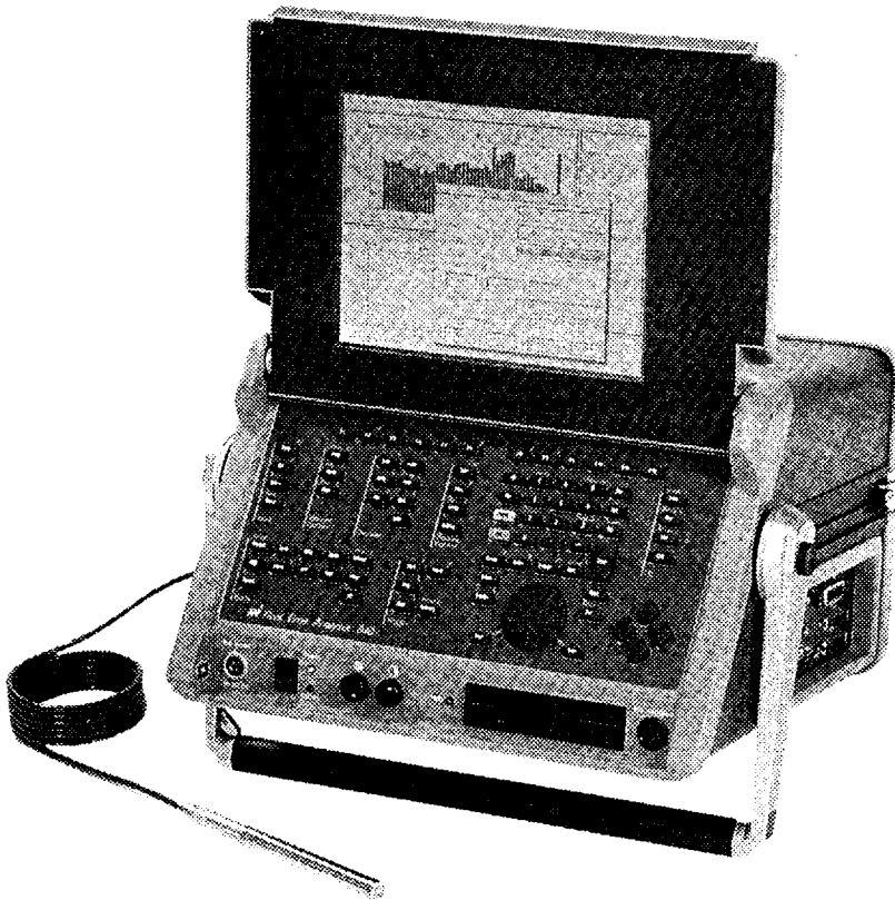
FIGURE 27.11 Real-time frequency analyzer for acoustic measurements.
