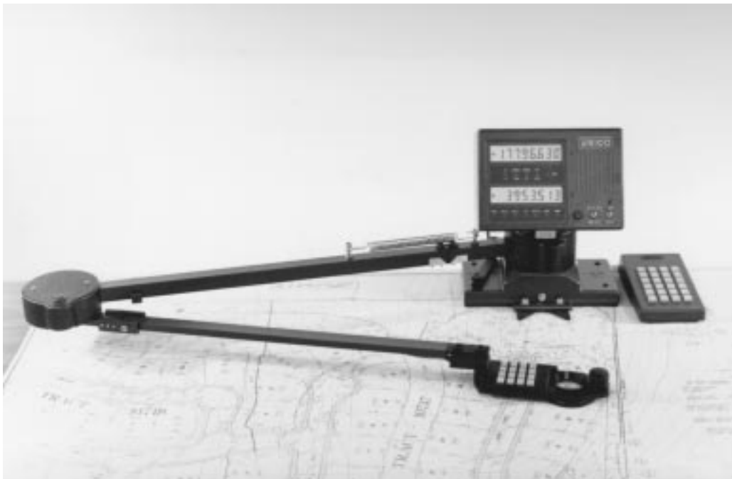
FIGURE 12.9 An arm digitizer lets one measure area, length, and coordinates, and transmit the displayed data to a computer; it requires minimum desk space.
