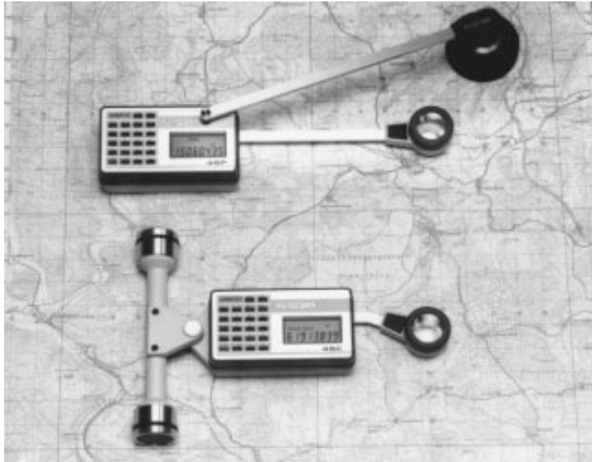
FIGURE 12.8 Battery-operated planimeters have the advantages of electronics planimeters and are portable.
