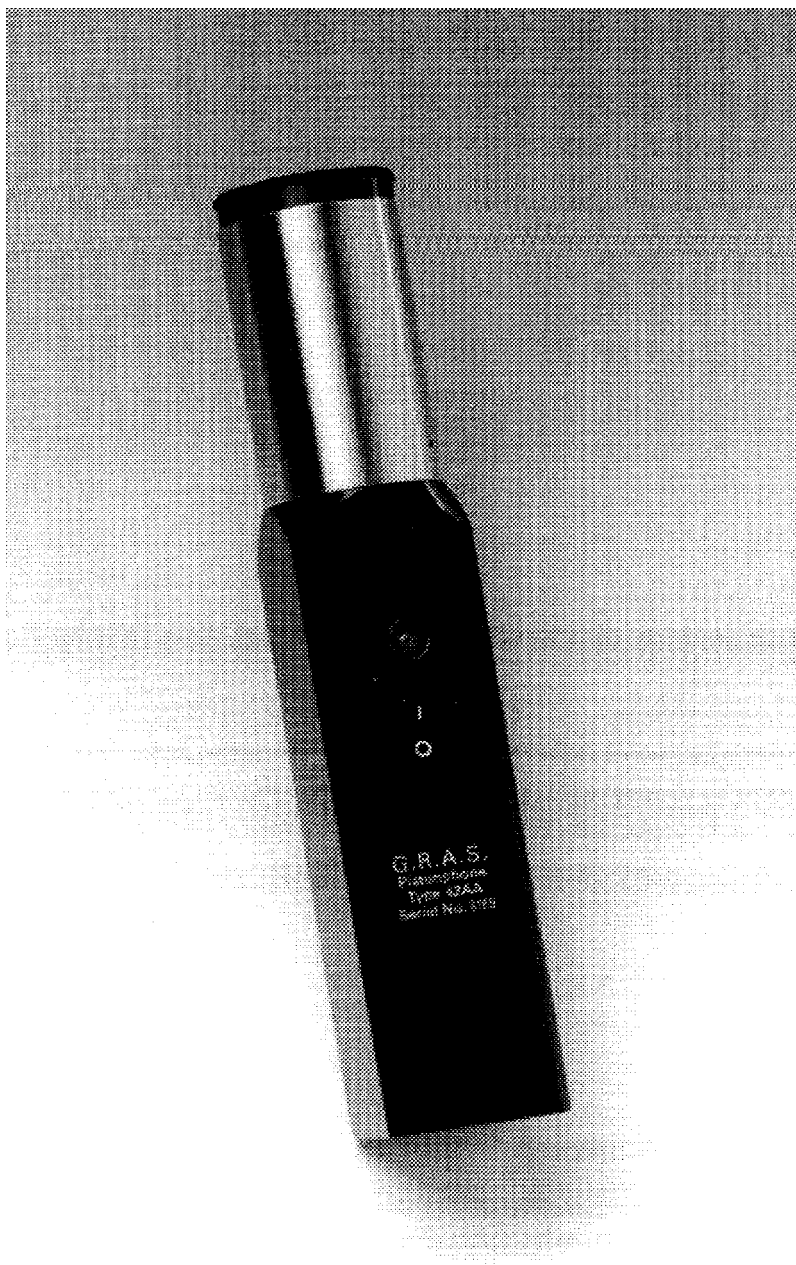
FIGURE 27.20 Pistonphone for microphone calibration.
