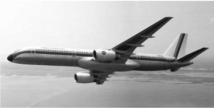
FIGURE 2.6 A Boeing 757-200 aircraft showing fairings under the wing. (Reprinted from 3DScanCo/GKS Global Services. With permission.)
