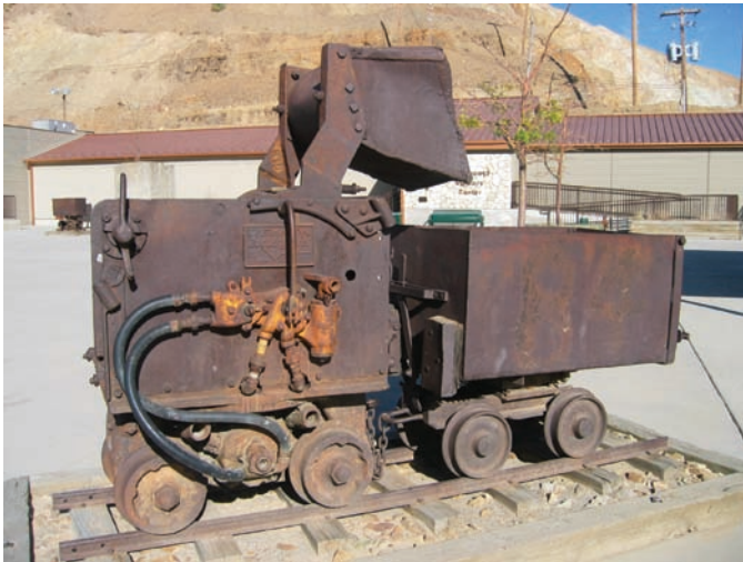
FIGURE 4.19 General corrosion observed on a mining cart.
