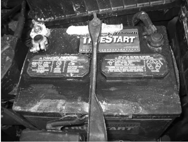
FIGURE 4.18 (See color insert following p. 142.) Corrosion due to electrochemical reaction.
