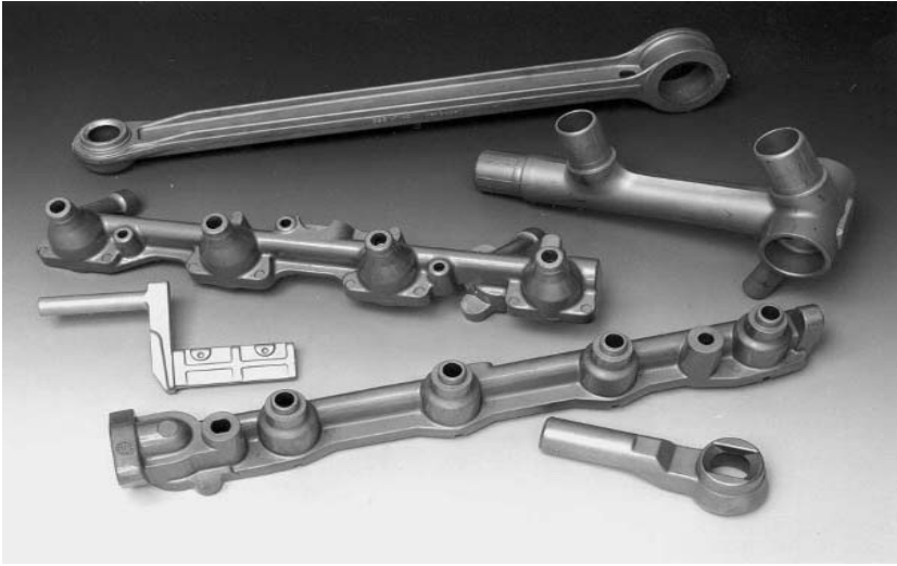
Figure 5.17 Automotive components manufactured using semi-solid metalworking processes. (Courtesy of Formcast, Inc.)
