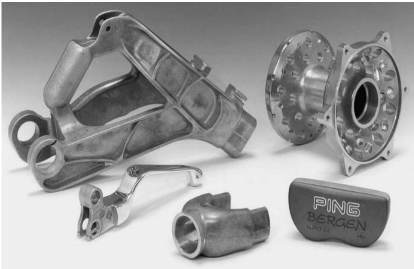
Figure 5.18 Components manufactured using semi-solid metalworking processes. (Courtesy of Formcast, Inc.)
