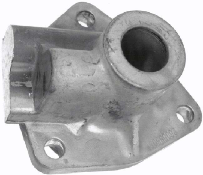
Figure 4.8 Squeeze cast valve housing. (Courtesy of SPX Contech Corporation.)
