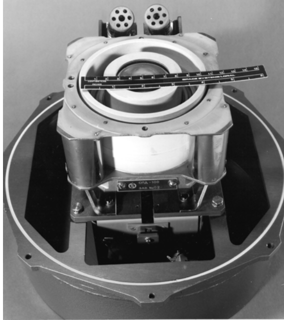
Figure 6.17. The Russian SP-100 Hall effect thruster. 100 mm diameter of the insulated cavity is shown by a ruler. The twin electron guns can be seen as well as two of the four coils that power the outer ring magnet. This is an SPT rather than a TAL device, it has a deep discharge cavity, insulated with boron nitride.
