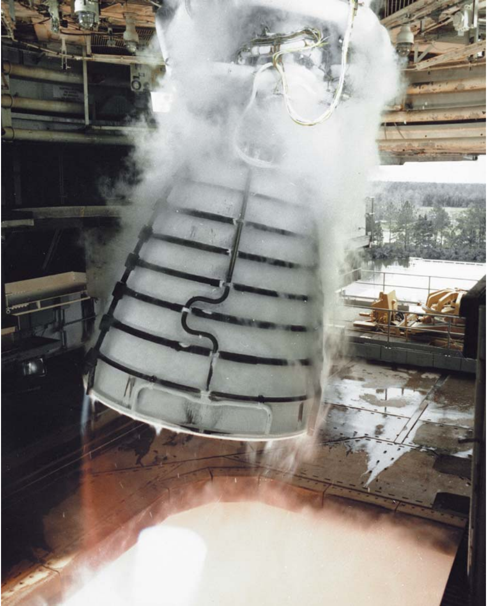
Plate 9 Testing the thrust vector control system on a Space Shuttle main engine while firing. Courtesy NASA.
