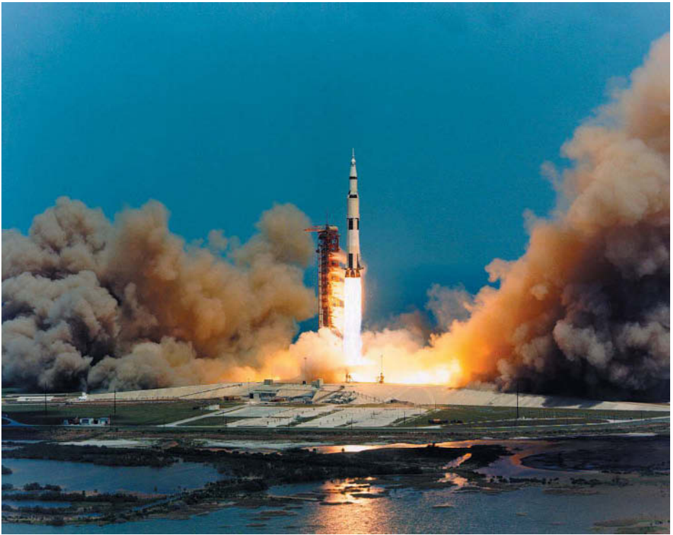
Plate 6 The launch of Apollo 16 on the Saturn V rocket. The five F1 liquid oxygen–kerosene engines produce a combined thrust of 34 MN to lift the Saturn V off the launch pad.
