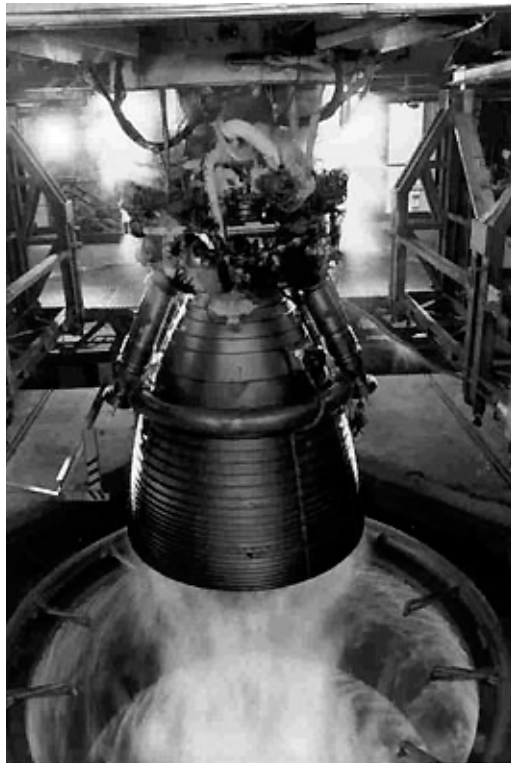
Figure 3.8. The Vulcain 2 under test. This is the new version of the Vulcain specified for Ariane 5. It uses a more oxygen-rich mixture to improve the mass ratio, and a longer nozzle to restore the exhaust velocity.
