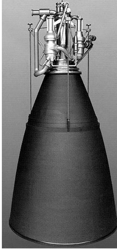
Figure 3.7. The Vinci cryogenic upper-stage engine. Note the very long nozzle extension to give the high exhaust velocity; it is deployed after separation of the main stage. This new cryogenic engine is specified for the updated Ariane 5, which will have a 10 tonne capacity to GTO.
