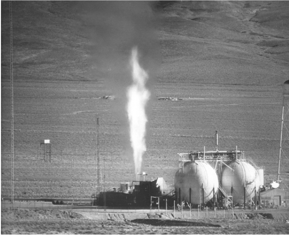
Figure 7.1. Actual test of a nuclear rocket engine at Jackass Flats in Nevada, as part of the NASA NERVA programme. The engine is firing vertically upwards, the storage tanks are for the liquid hydrogen.
