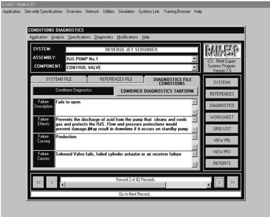
Fig. 3.68 Hazards criticality analysis component condition
