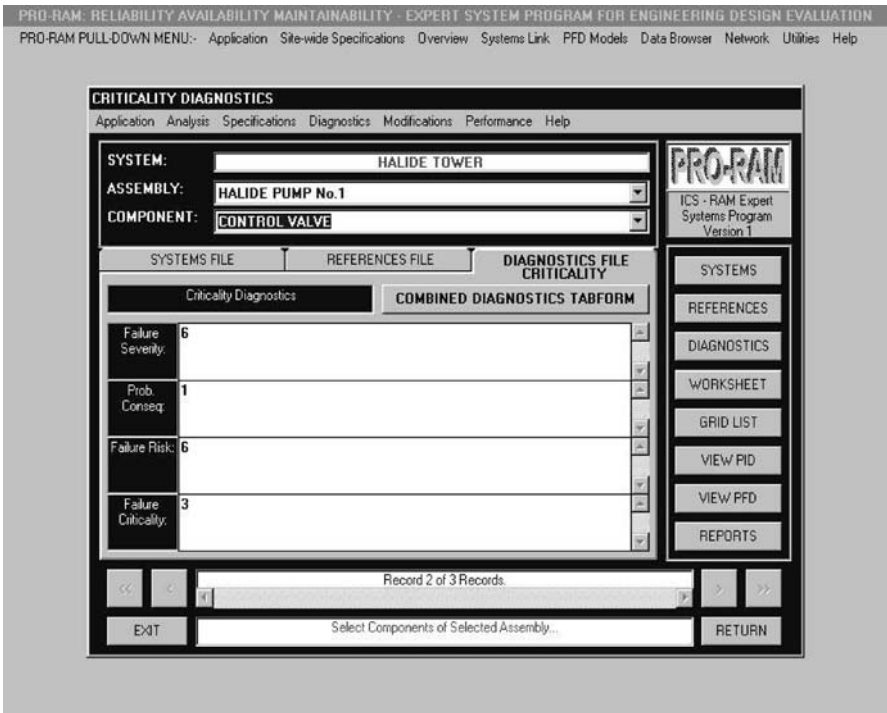
Fig. 5.112 Determining the criticality of consequences of failure
