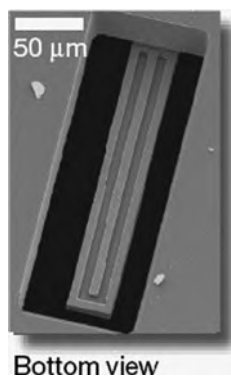
Fig. 1.38 (a) Electron micrograph of a suspended microchannel resonator. The 200\ \mu\text{m} \times 33\ \mu\text{m} \times 7\ \mu\text{m} (length \times width \times thickness) microcantilever containing a 3\ \mu\text{m} \times 8\ \mu\text{m} (height \times width) channel is suspended in a vacuum cavity. The cantilever has been intentionally etched open to visualize the fluidic conduit inside. (Reprinted with permission from [1.153]. © 2007 Nature Publishing Group)
