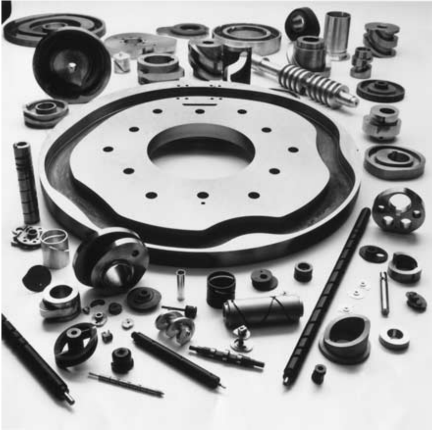
FIGURE 1.6. Various types commercial of cams. (Courtesy Commercial Cam Co., Inc., Wheeling, Ill.)
