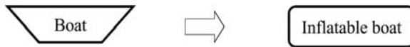
Figure 10.30 Principle 29: Pneumatics and hydraulics. Use gas and liquid instead of solid parts.
