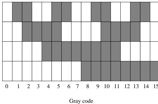
Figure 10.8 Gray code pattern corresponding to Table 10.1.
