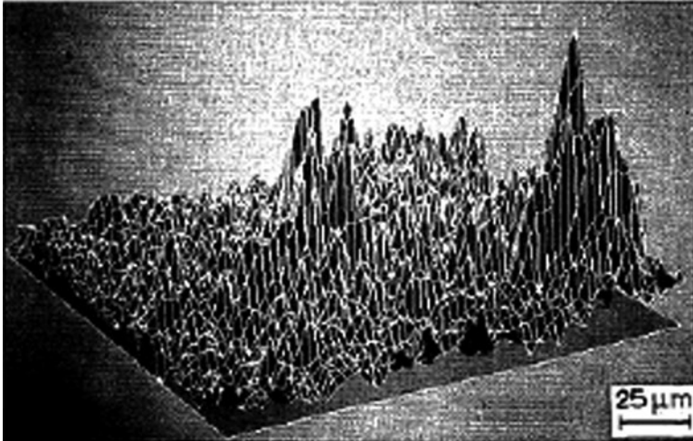
Fig. 8.25 Intensity distribution of carbon in an area on tribosurface
