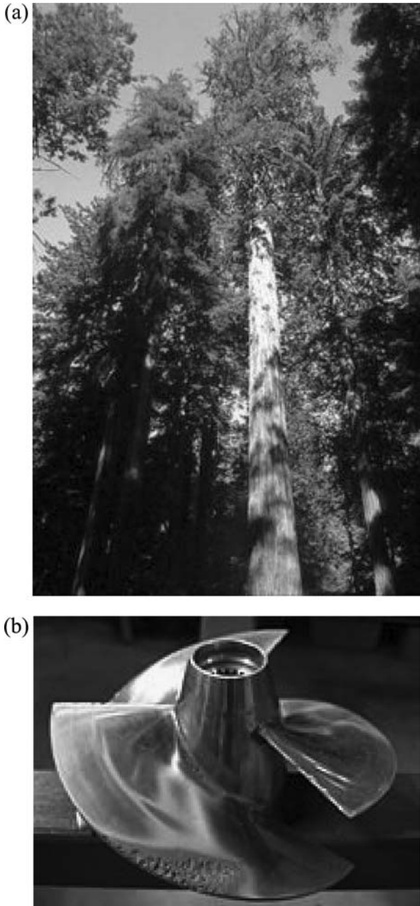
Fig. 5.4. Effect of negative water pressure in everyday life. a California Redwood (Sequoia) is an example of a tall tree which needs to develop a negative pressure in order to suck water from the roots up to the top. b Cavitation damage of a boat propeller. A rapid rotation of the propeller leads to water pressure decrease and cavitation (bubbling) that can damage to propeller over a long period of time
