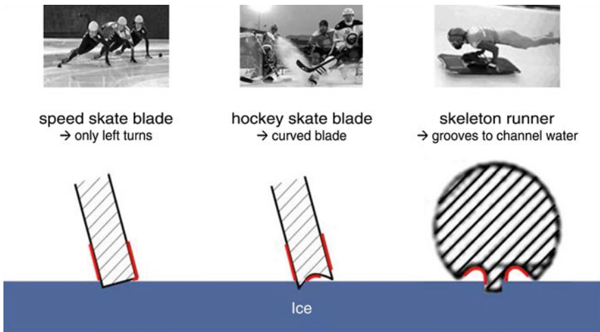
Fig. 9.23 Examples for non-load-bearing surfaces of ice sports blades, which rendered hydrophobic will assist to reduce friction on ice
