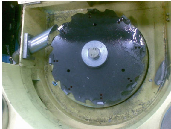
Fig. 20.19 Edge milling of cast Alu plate on casting machine
