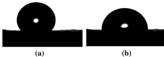
Fig. 6.4 Wetting transitions observed by vibration of 15 \mu\text{l} water drop deposited on the micrometrically rough PDMS surface. a The initial Cassie state. b The Cassie impregnating state induced by vibrations
