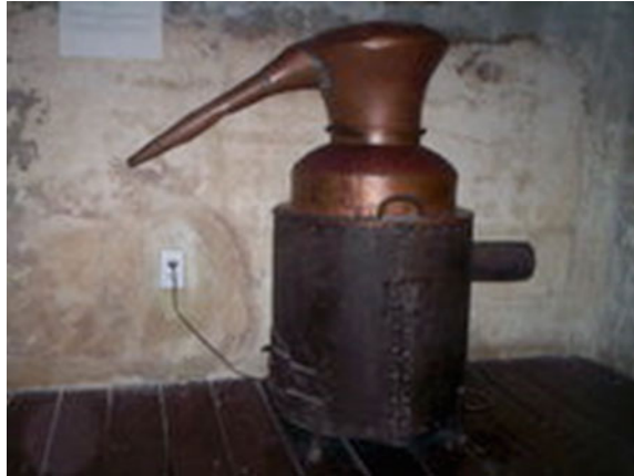
Fig. 19.5 Ship desalination device using distillation. Kura-Hulanda Museum, Willemstad, Curacao, Netherlands Antilles (photo by M. Nosonovsky 2005)
