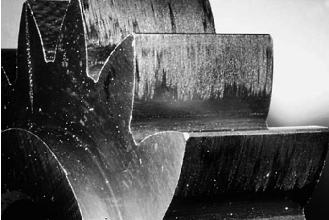
Fig. 18.22 Gear tooth surfaces with scuffing damage, from [67]
