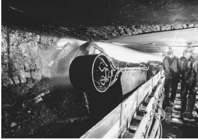
A longwall shearer cuts swatches of coal 750 feet long and 28 inches thick, 800 feet underground at Consolidation Coal Company's Blacksville #2 mine. (Corbis-Bettmann)
