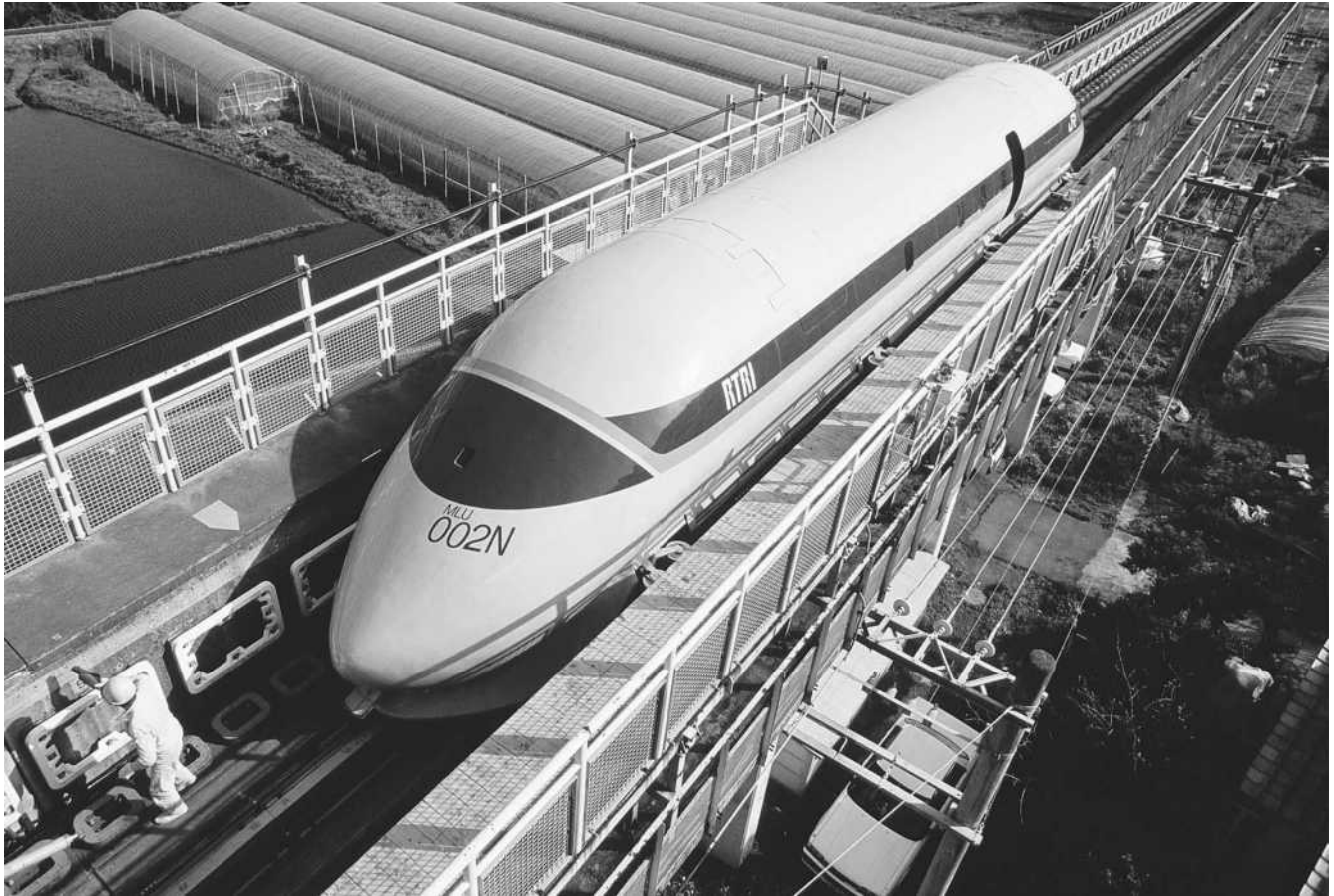
A train that operates by magnetic levitation, at a railroad research center in Japan. (Corbis-Bettmann)
