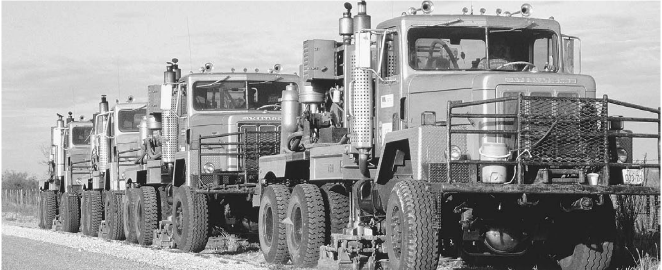
This is a team of trucks that create and record seismic vibrations, in an attempt to detect the presence of oil. (Corbis Corporation)
