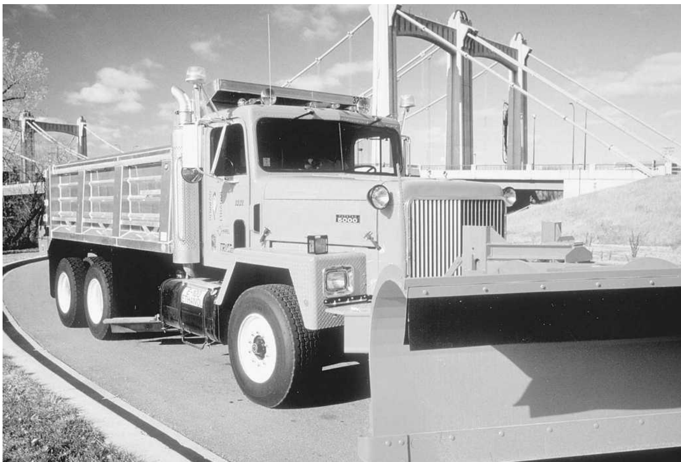
Ethanol-powered snowplow in Hennepin County, Minnesota. (U.S. Department of Energy)
