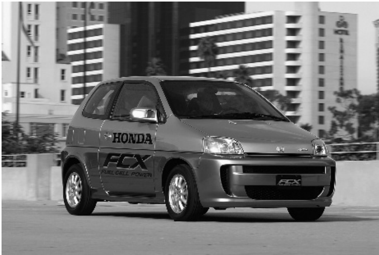
Figure 1.15 The Honda FCX was the first fuel cell car to be certified for use by the general public in the USA in 2002, and so theoretically become publicly available. This four seater city car has a top speed of 150kph and a range of 270km. The hydrogen fuel is stored in a high-pressure tank (Photograph reproduced by kind permission of Ballard Power Systems.)
