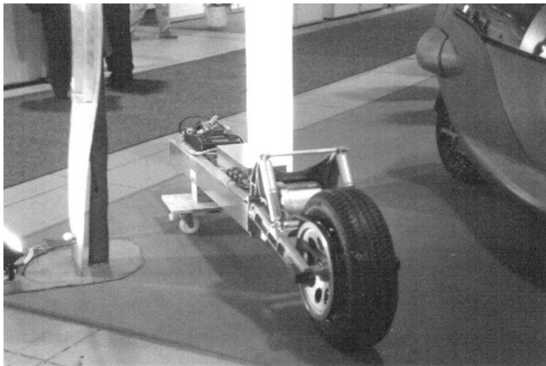
Figure 8.11 This power module comprises motor, controller, battery and one driven wheel in a neat unit that could be built into a wide range of vehicle designs
