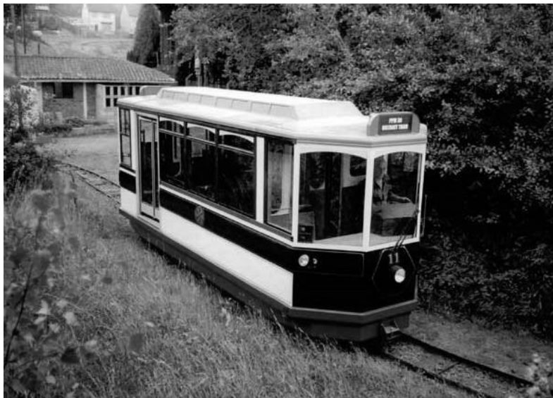
Figure 1.17 The Parry People Mover. This electric vehicle uses a flywheel to store energy (Photograph kindly supplied by Parry People Movers Ltd.)
