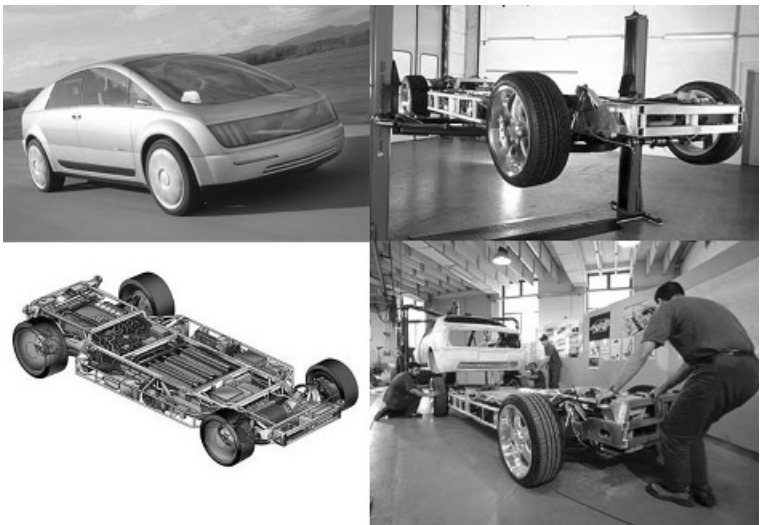
Figure 8.16 General motors Hy-wire chassis (Reproduced by kind permission of General Motors Corp.)
