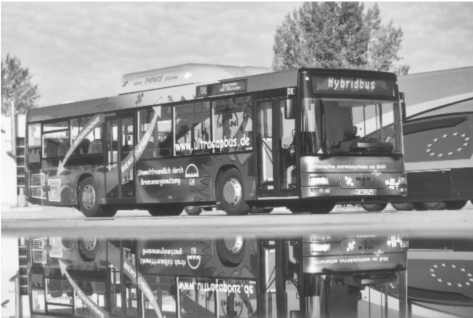
Figure 1.18 Hybrid diesel/electric bus, with electrical energy stored in capacitors (Photograph reproduced by kind permission of Man Nutzfahrzeuge AG.)
