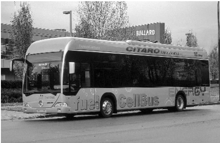
Figure 1.16 Citaro fuel cell powered bus, one of a fleet entering service in 2003 (Photograph reproduced by kind permission of Ballard Power Systems.)
