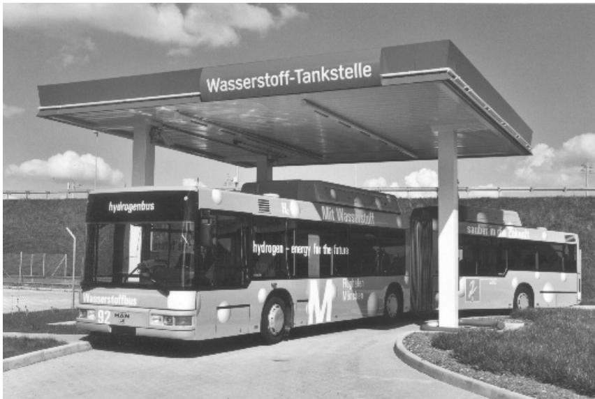
Figure 5.2 A hydrogen filling station. The bus in the picture is not electric, but uses a hydrogen fuelled IC engine (picture kindly supplied by MAN Nutzfahrzeuge A.G.)
