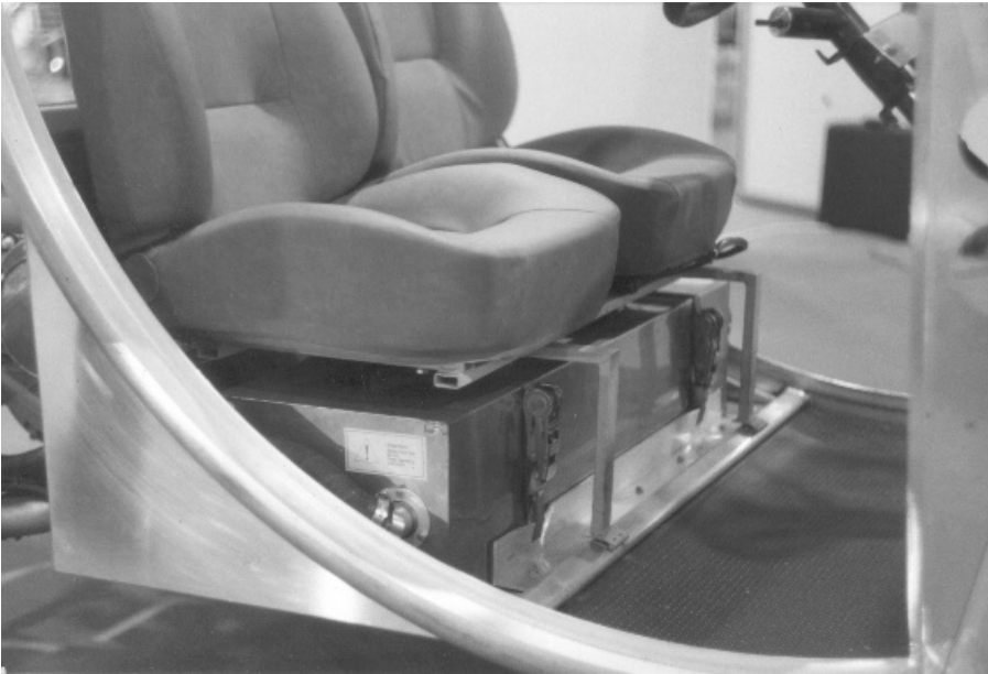
Figure 2.11 A commercial Zebra battery fitted neatly under the seat of an experimental battery electric vehicle by MES-DEA. The battery stores about 18 kWh of electrical energy
