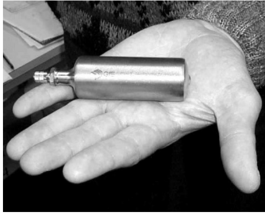
Figure 5.5 Metal hydride stores can be made quite small, as this example shows
