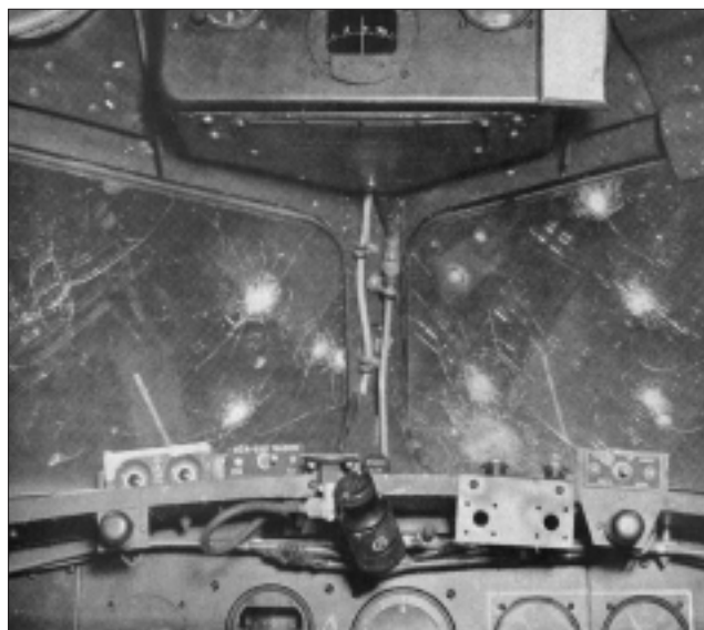
Flak-Damaged B-17 Windshield
