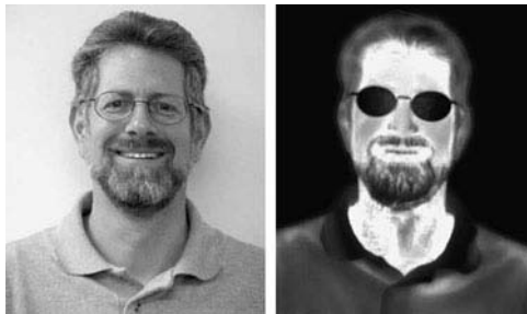
Fig. 3.47 Photographs in visible light and IR thermal radiation that is naturally emanated from the object. Note the brighter (appearing warmer) areas at the wrinkles and skin folds near the nose - a result of the cavity effect. Eyeglasses appear black (cold) because glass is opaque in the mid- and far infrared spectral ranges and does not pass thermal radiation (photo courtesy of Infrared Training Center, www.infraredtraining.com )
