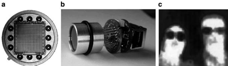
Fig. 14.21 Thermopile thermal-imaging sensor: sensing surface (a); imaging module (b); and example of a thermal image (c) (courtesy of Heimann Sensors, www.heimannsensors.com )
