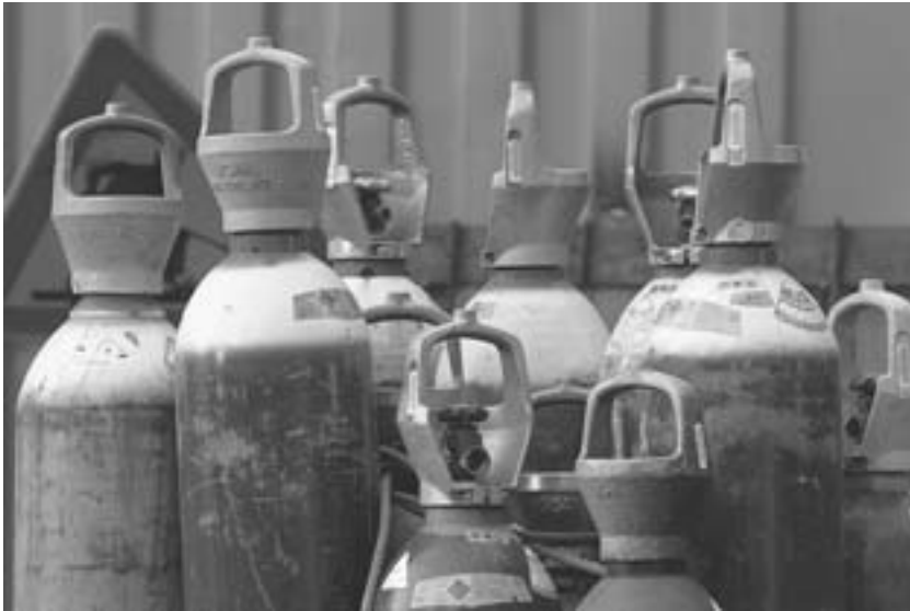
FIGURE 3.5 Improper storage of oxygen and acetylene cylinders
