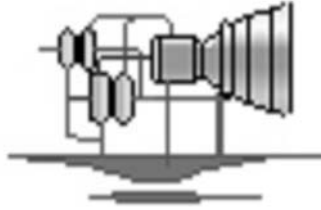
Figure 4.20. Integrated ejector ram-scamjet rocket.
