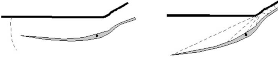
Figure 4.12. Variable capture area, inward-turning inlet.
