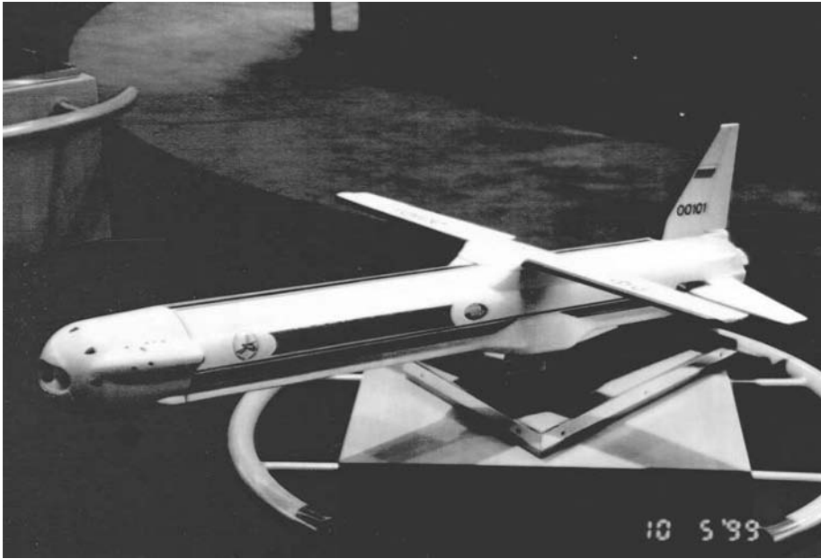
Figure 2.12. Fly-back version of the strap-on as an alternative to lifting parachutes.
