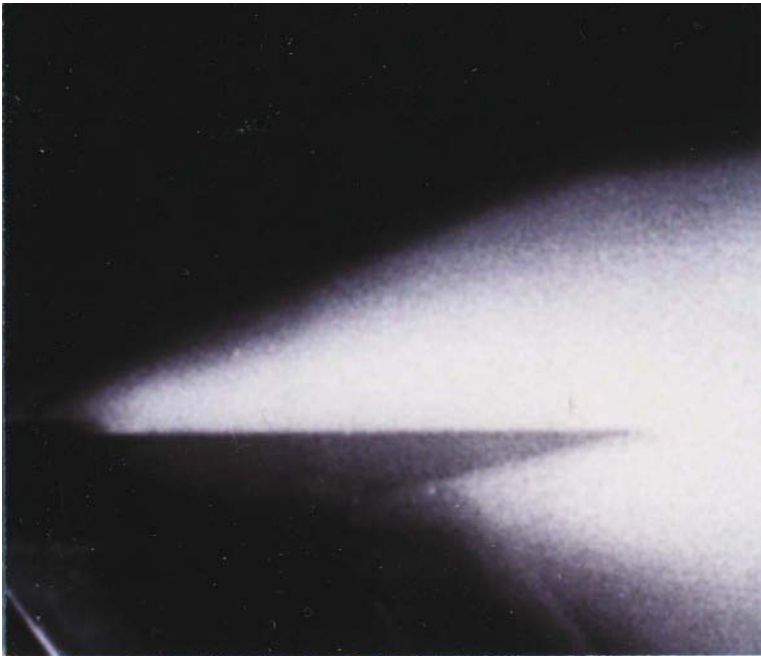
Figure 4.21. 300°C hydrogen injected into supersonic air stream at flight conditions corresponding to a scramjet combustor for an aircraft flying at Mach 8. Tests circa 1962.
