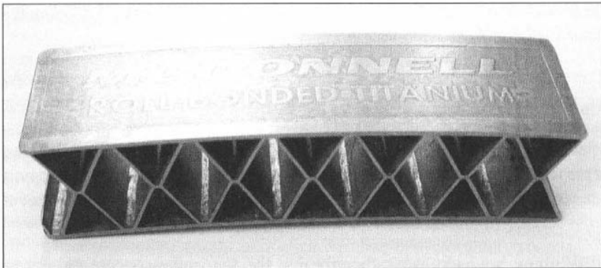
Figure 3.18. McDonnell Aircraft Company Roll-Bonded Titanium Structure (circa 1963), from Advanced Engine Development at Pratt & Whitney SAE [Mulready, 2001]. Today this structure would be super-plastically formed and diffusion-bonded from RSR titanium sheets.
