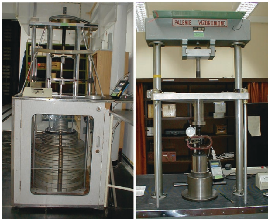
Fig. 5 Machines used for calibration of force patterns, on the left – a machine with the range 0–60,000 N, on the right – a machine with the range 0–5,000 N, the picture was taken in 2008
