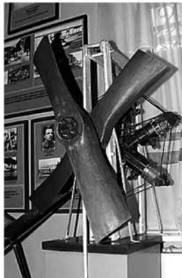
Fig. 4. General view of the birotative engine; diameter 1 m, length 0.85 m, weight 50 kg, average power 18 kW.
