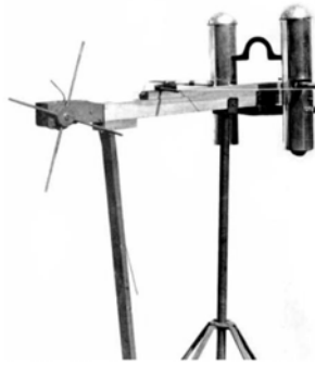
Fig. 13. The cheiroballista as reconstructed by E. W. Marsden (Lahanas, Web).
