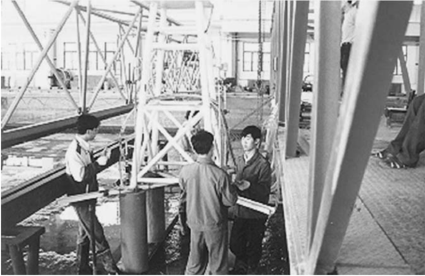
Figure 14.9 A 4-bucket foundation model platform prepared for a penetration test into the model ocean
