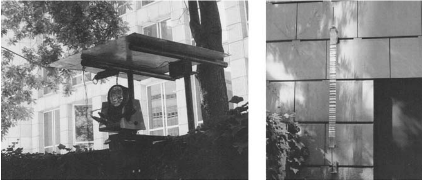
Figure 12.10 Motorized digital levelling device (left) and levelling board (right)
