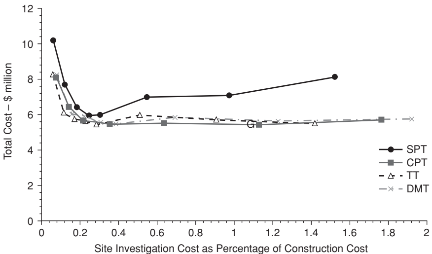
Figure 1.14 Expected total cost based on a site investigation consisting of samples arranged in an RG pattern and reduced using the SA on a soil with a COV of 50% and SOF of 8 m
