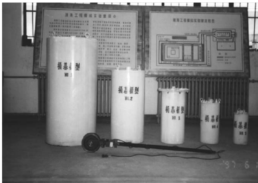
Figure 14.8 Model buckets used in the laboratory single bucket penetration tests. The buckets are constructed with 5 mm-thick steel sheet
