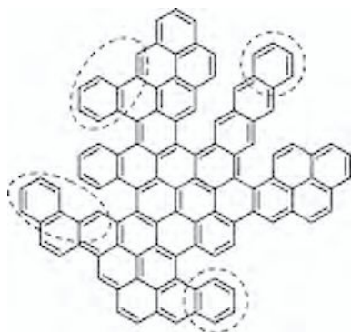
Figure 4. A computed PAH molecule after a simulation time of 0.1 ms. The combined sites involving three adjacent free-edges (R6 ring) are shown inside circles. The combined sites involving an R6 ring next to an armchair (R6 AC) are shown inside ellipses.
