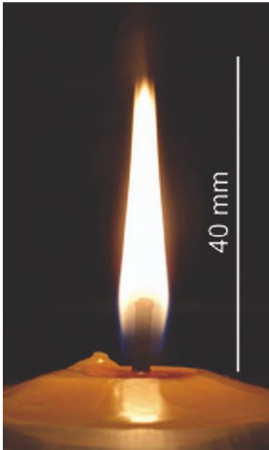
Figure 1. Color image of a candelilla candle flame at its smoke point. This smoke point is 37.0 mm, the wick diameter is 1.7 mm, and the wick length is 9.3 mm. These dimensions are slightly different from the mean values reported elsewhere in this manuscript.
